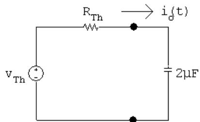
$$v_{Th} = \frac{5}{6}v_g; \quad R_{Th} = 60\parallel 12 = 10 \text{ k}\Omega$$
