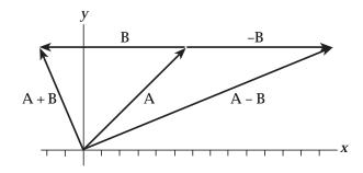
3.7 (a) In your vector diagram, place the tail of Vector  $\mathbf{B}$  at the tip of Vector  $\mathbf{A}$ . The vector sum,  $\mathbf{A} + \mathbf{B}$ , is then found as shown in the vector diagram and should be
