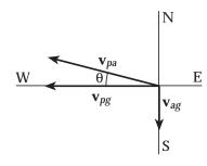
$\mathbf{v}_{pg}$  = the velocity of the plane relative to the ground (to be due west).
