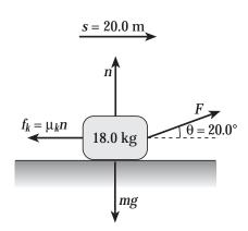
$$F = \frac{\mu_k mg}{\mu_k \sin \theta + \cos \theta} = \frac{(0.500)(18.0 \text{ kg})(9.80 \text{ m/s}^2)}{(0.500)\sin 20.0^\circ + \cos 20.0^\circ} = \boxed{79.4 \text{ N}}$$
