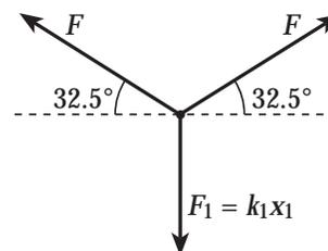
If  $F = 210 \text{ N}$  and  $k_1 = 5.60 \times 10^4 \text{ N/m}$ , the elongation of the spring is
