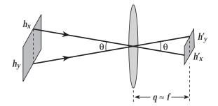
the image is  $h'_{y} = q\theta$ , or  $h'_{y} \propto q$ . Similarly for the horizontal dimension,  $h'_{x} \propto q$ , and the area of the image is  $A_{\text{in age}} = h'_{x}h'_{y} \propto q^{2}$ . Assuming a very distant object,  $q \approx f$ , so  $A_{\text{in age}} \propto f^{2}$  and we conclude that  $I \propto 1/f^{2}$ .
