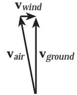
(b) For the return flight along path I,  $\mathbf{v}_{ground} = \mathbf{v}_{air} + \mathbf{v}_{wind}$  gives
