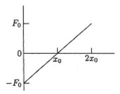
Since the area of a triangle is (base)(altitude)/2, the work done from x = 0 to  $x = x_0$  is  $-(x_0)(F_0)/2$  and the work done from  $x = x_0$  to  $x = 2x_0$  is  $(2x_0 - x_0)(F_0)/2 = (x_0)(F_0)/2$ . The total work is the sum, which is zero.
