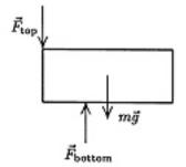
80. When the log is on the verge of moving (just before its left edge begins to lift) we take the system to be in equilibrium with the static friction at its maximum value  $f_{s,\text{max}} = \mu_s F_N$ . Thus, our force and torque equations yield
