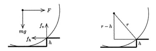
We calculate the torque around the step corner. The second diagram indicates that the distance from the line of F to the corner is r - h, where r is the radius of the wheel and h is the height of the step.
