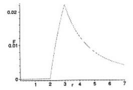
(b) Starting with the large r formula for force, we integrate and obtain the expected U = -GmM/r (for  $r \ge a$ ). Integrating the force formula indicated above for  $b \le r \le a$  produces
