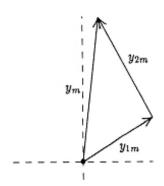
34. The phasor diagram is shown below. We use the cosine theorem:
