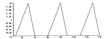
(d) The leading edge of the pulse reaches x = 10 cm at t = (10 - 4.0)/5 = 1.2 s. The particle (say, of the string that carries the pulse) at that location reaches a maximum displacement h = 2 cm at t = (10 - 3.0)/5 = 1.4 s. Finally, the trailing edge of the pulse departs from x = 10 cm at t = (10 - 1.0)/5 = 1.8 s. Thus, we find for h(t) at x = 10 cm (with the horizontal axis, t, in seconds):
