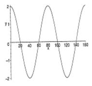
(c) The wave can be written as  $y(x,t) = y_m \sin(kx + \omega t)$ , where  $v = \omega/k$  is the speed of propagation. From the problem statement, we see that  $\omega = 2\pi/0.40 = 5\pi$  rad/s and  $k = 2\pi/80 = \pi/40$  rad/cm. This yields  $v = 2.0 \times 10^2$  cm/s = 2.0 m/s
