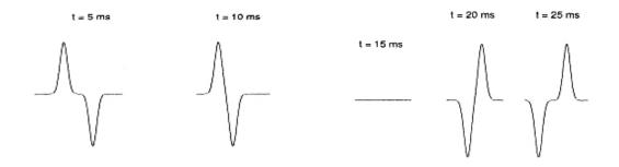
(b) The particles of the string are moving rapidly as they pass (transversely) through their equilibrium positions; the energy at t = 15 ms is purely kinetic.
