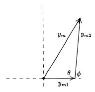
$$\cos\phi = \frac{y_m^2 - y_{m1}^2 - y_{m2}^2}{2y_{m1}y_{m2}} = \frac{(9.0 \,\text{mm})^2 - (5.0 \,\text{mm})^2 - (7.0 \,\text{mm})^2}{2(5.0 \,\text{mm})(7.0 \,\text{mm})} = 0.10.$$
