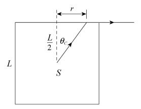
Light leaving the source at a small angle  $\theta$  is refracted at the face and leaves the cube; light leaving at a sufficiently large angle is totally reflected. The light that passes through the cube face forms a circle, the radius r being associated with the critical angle for total internal reflection. If  $\theta_c$  is that angle, then
