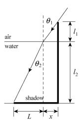
Here  $\theta_1 = 90^\circ - \theta = 35^\circ$ ,  $\ell_1 = 0.50$  m, and  $\ell_2 = 1.50$  m. The length of the shadow is x + L. x is given by
