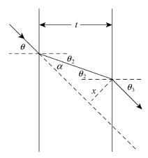
The emerging ray is parallel to the incident ray. We wish to derive an expression for x in terms of  $\theta$ . If D is the length of the ray in the glass, then  $D \cos \theta_2 = t$  and  $D = t/\cos \theta_2$ . The angle  $\alpha$  in the diagram equals  $\theta - \theta_2$  and  $x = D \sin \alpha = D \sin (\theta - \theta_2)$ . Thus
