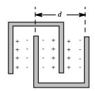
When there are two plates in each comb, the number of adjoining sheets of positive and negative charge is 3, as shown in the sketch. When there are N plates on each comb, the number of parallel capacitors is 2N-1 and the total capacitance is
