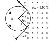
$F_B = qvB = \frac{mv^2}{R}$  so  $R = \frac{mv}{qB} = \frac{(1.67 \times 10^{-27} \text{ kg})(3.39 \times 10^7 \text{ m/s})}{(1.60 \times 10^{-19} \text{ C})(1.00 \text{ T})} = 0.354 \text{ m}$
