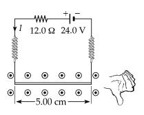
$$F_{\text{magnetic}} = 2 \left( \frac{mg}{2\Delta x_1} \right) \Delta x_2 = \frac{mg \Delta x_2}{\Delta x_1}; \quad \text{but} \quad |\mathbf{F}_B| = I |\mathbf{L} \times \mathbf{B}| = ILB$$
