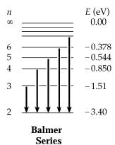
(b) The biggest energy loss is for an electron to fall from ionization,  $n = \infty$ , to the n = 2 state.
