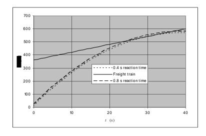
Remarks: A collision occurs the first time the curve for the passenger train crosses the curve for the freight train. The smaller of two solutions will always give the time of the collision.
