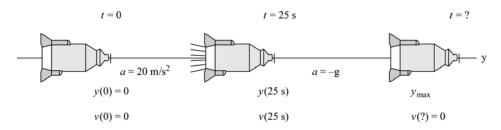
(a) Express the highest point the rocket reaches, h, as the sum of its displacements during the first two stages of its flight:
