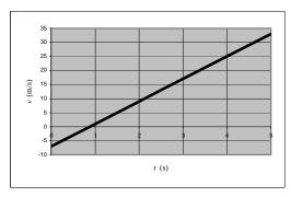
The instantaneous acceleration is defined as the time derivative of the velocity or the slope of the velocityversus-time curve:
