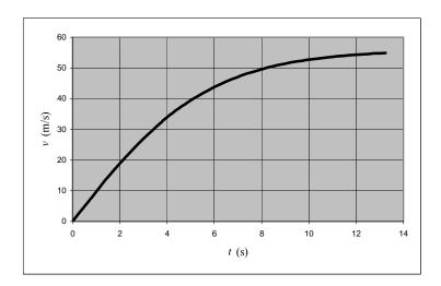
Note that the velocity increases linearly over time (i.e., with constant acceleration) for about time *T*, but then it approaches the terminal velocity as the acceleration decreases.
