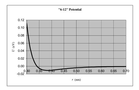
(b) The minimum value is about -0.0107 eV, occurring at a separation of approximately 0.380 nm. Because the function is concave upward (a potential "well") at this separation, this separation is one of stable equilibrium, although very shallow.
