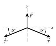
(a) Noting that, due to symmetry, T' = T, apply  $\sum F_y = 0$  to the string at the point of contact with the bridge:
