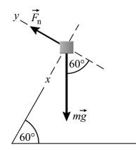
From the free - body diagram, we see that the forces acting on the block are a gravitational force that acts downward and the normal force that the incline exerts perpendicularly to the incline.
