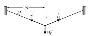
(a) Use trigonometry to relate the sag s in the rope to its length L and  $\theta$ :
