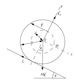
The spool will move down the plane at constant acceleration, spinning in a counterclockwise direction as string unwinds.
