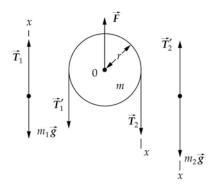
(a) Apply Newton's 2<sup>nd</sup> law to the pulley and the two objects:
