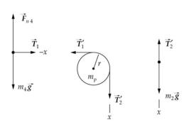
Apply Newton's 2<sup>nd</sup> law to the two blocks and the pulley:
