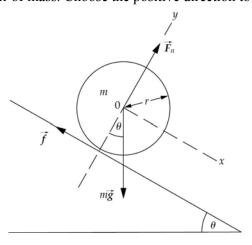
Apply  $\sum \vec{F} = m\vec{a}$  to the thin spherical shell:
