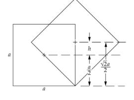
Express the work done in moving the cube a distance a by raising its center of mass from y = a/2 to  $y = \sqrt{2}a/2$  and then letting the cube flop down:
