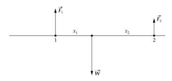
The stick remains balanced as long as the center of mass is between the two fingers. For a balanced stick the normal force exerted by the finger nearest the center of mass is greater than that exerted by the other finger. Consequently, a larger static - frictional force can be exerted by the finger closer to the center of mass, which means the slipping occurs at the other finger.
