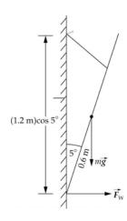
(a) Because the center of gravity of the picture is in front of the wall, the torque due to mg about the nail must be balanced by an opposing torque due to the force of the wall on the picture, acting horizontally. So that  $\sum F_x = 0$ , the tension in the wire must have a horizontal component, and the picture must therefore tilt forward.
