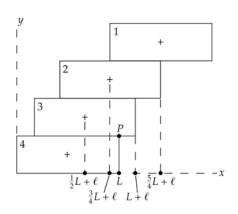
(a) Apply  $\sum \vec{\tau} = 0$  about an axis through P and parallel to the z axis to bricks 1 and 2 for the 3-brick arrangement shown above on the left:
