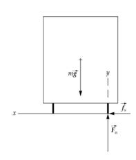
Apply  $\sum \vec{\tau} = 0$  about an axis through the center of gravity of the
