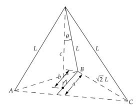
Letting  $F_{\rm C}$  represent the compressional force in a leg of the tripod, apply  $\sum \vec{F} = 0 \text{ to the apex of the tripod:}$
