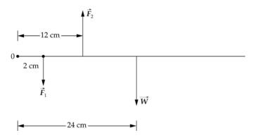
(a) Letting the upward force exerted by the fencer's hand be F, apply  $\sum F_y = 0$  to the epee to obtain:
