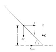
To find the force required to pull the ladder away from the wall, apply  $\sum \vec{\tau} = 0$  about an axis through the bottom of the ladder:
