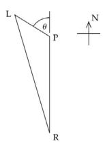
Using the law of cosines, relate the angle  $\theta$  to the distances that make up the sides of the triangle:
