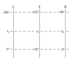
Referring to the diagram, set up a proportion to convert temperatures on the Réaumur scale to Celsius temperatures:
