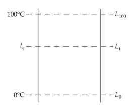
$$\frac{t_{c} - 0^{\circ}\text{C}}{100^{\circ}\text{C} - 0^{\circ}\text{C}} = \frac{L_{t} - L_{0}}{L_{100} - L_{0}}$$
