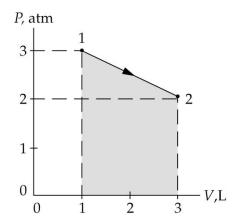
The work done by the gas equals the area under the curve:
