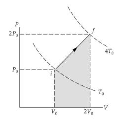
The work done by the gas equals the area under the curve:
