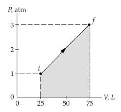
The work done by the gas equals the area under the curve:
