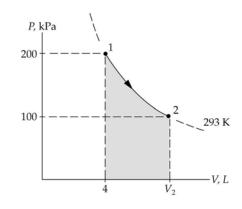
$$W_{\text{by gas}} = \int_{V_1}^{V_2} P dV = nRT \int_{V_1}^{V_2} \frac{dV}{V} = P_1 V_1 \int_{V_1}^{V_2} \frac{dV}{V}$$
