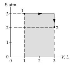
The work done by the gas equals the area under the shaded curve:
