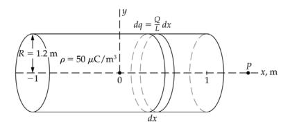
Express the electric field on the x axis due to the charge carried by the disk of thickness dx:
