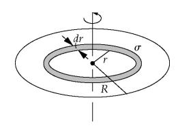
Applying Ampere's law to a circular current loop of radius *r* we obtain:
