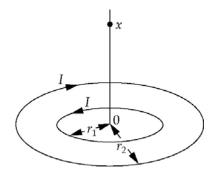
$$B_1 = \frac{\mu_0}{4\pi} \frac{2\pi r_1^2 I}{\left(x^2 + r_1^2\right)^{3/2}} = \frac{\mu_0 r_1^2 I}{2\left(x^2 + r_1^2\right)^{3/2}}$$
