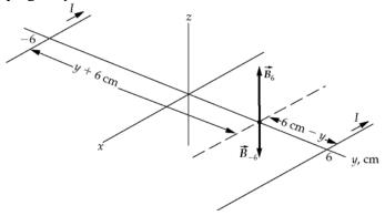
The field due to the current in the wire located at y = 6 cm is:
