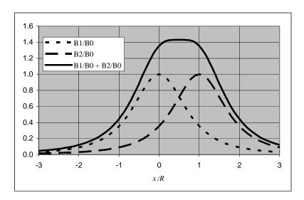
Note that, midway between the two loops, dB(x)/dx = 0. Also, when d = R, B(x) is nearly flat at the midpoint which shows that in the region midway between the two coils B(x) is nearly constant.
