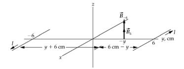
The field due to the current in the wire located at y = 6 cm is:
