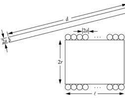
The self-inductance of an inductor with length  $\ell$ , cross-sectional area A, and number of turns per unit length n is:
