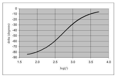
Referring to the spreadsheet program, we see that when  $f = f_{3 \text{ dB}}$ ,  $\delta \approx \boxed{-44.9^{\circ}}$ . This result is in good agreement with its calculated value of  $-45.0^{\circ}$ .
