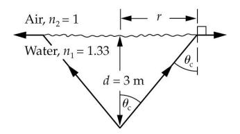
Relate the radius of the circle to the depth d of the point source and the critical angle  $\theta_c$ :
