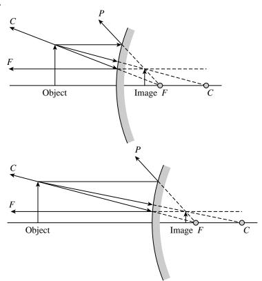
From the ray diagrams, we see that the image increases in size as the object is brought closer to the mirror's surface.
