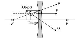
The image is located between the object and the lens, at about  $\frac{1}{3}|f|$ .
