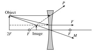
The image is located between the object and the lens, at about  $\frac{2}{3}|f|$ .
