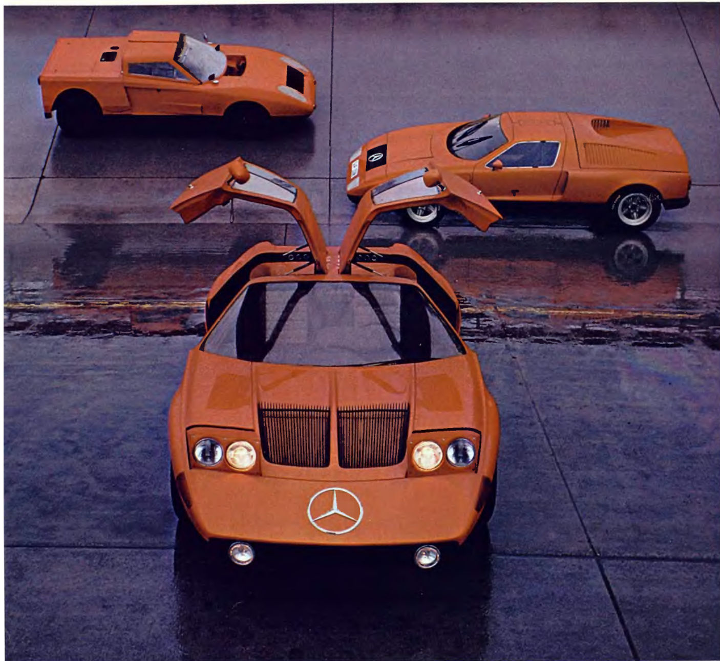
Three generations of the Wankel-powered Mercedes-Benz C-111. The original prototype is at upper left and the three-rotor, 160-mph version shown to the press in the summer of 1969 at middle right. Foreground, its awesome successor, the four-rotor, 400-horsepower, 186-mph model.
