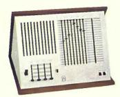
The Muse, a portable electronic computer that composes and plays music, is programmed with slide switches on front panel, by Triadex, \$300.
