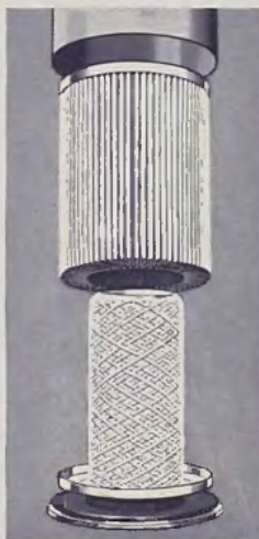
The outer filter: a 6 foot phenolic impregnated cellulose element. The inner filter: a fiber strand more than 60 feet long, wound on a steel core. Your oil goes through both approximately once every 30 seconds!
