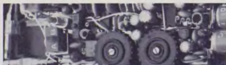
The PocketCom components are equivalent to 112 transistors whereas most comparable units contain only twelve.
