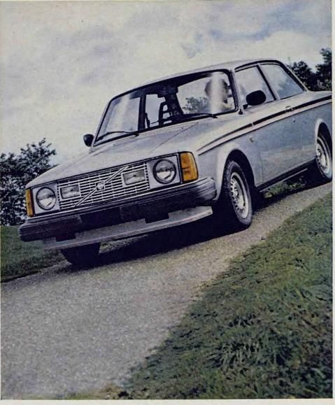
The 242GT is also built to keep you out of trouble. You get dual brake circuits with four power-assisted discs; a special valve on each rear brake line designed to minimize premature lock-up; and impact-absorbing front and rear ends surrounding a steel passenger cage to keep you out of really big trouble.
