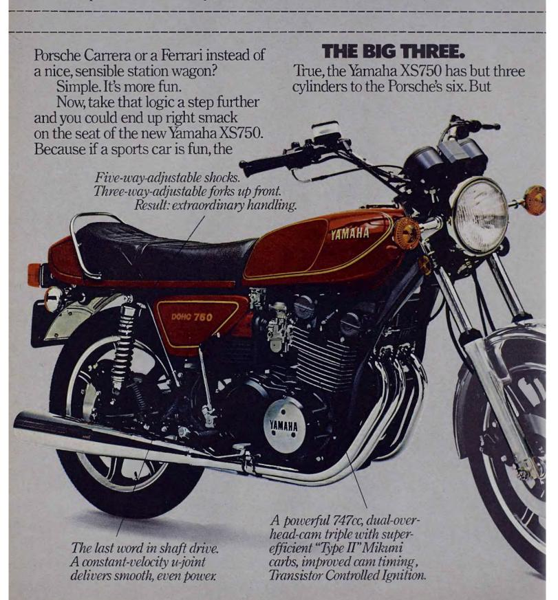
those three cylinders, ably assisted by dual overhead cams, electronic ignition and newly-designed "Type II" Mikuni carburetors give the 750 an incredible 9000 rpm redline.
