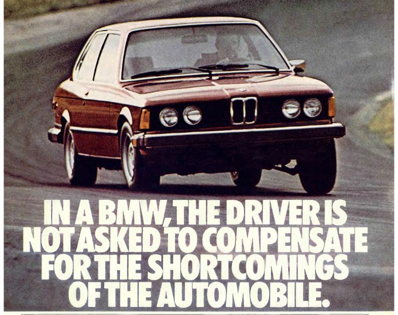
The extraordinary road-holding ability of the BMW 320i is graphically illustrated, above, travelling at a high speed through turn # 6 at the Sears Point International race course. Note: as the BMW goes into the turn, the unique angling of the MacPherson front struts reduces the lean of the inside front wheel, while the outside front wheel remains vertical; inside and outside rear wheels remain vertical due to semi-trailing arm design in the rear.
