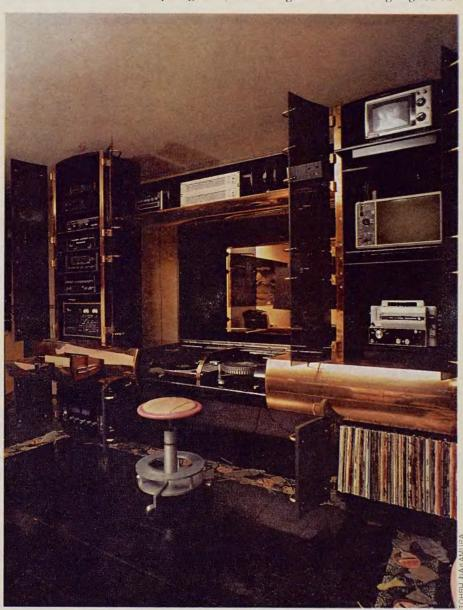
Left: This satellite section is a soundproof rolling projection booth that's capable of housing up to four projectors (an umbilical cord links the booth with the console's central control unit). The copper-fronted drawers are for storing a collection of films and slides.
