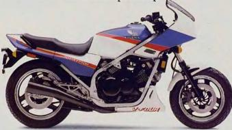
Now, you can ride the 1985 Interceptor, with a liquid-cooled 699cc DOHC 90° V-4 that develops an incredible 81° horsepower. A race-designed rectangular-section frame. Air-adjustable Pro-Link® rear suspension with adjustable damping. Triple-disc brakes and Honda's exclusive Torque Reactive Anti-dive Control (TRAC"). It's armed with more championship-technology than any other production machine.
