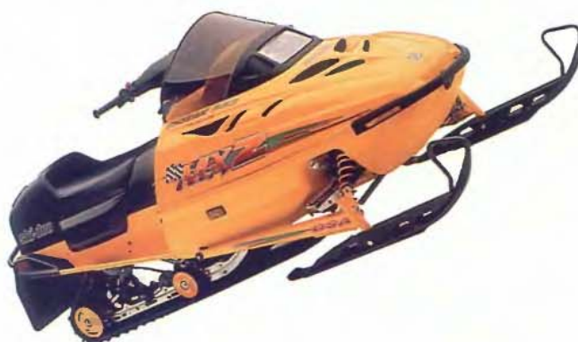
Named Sled of the Year by SnoWest magazine, Ski-Doo's aluminum-chassis MX Z 583 snowmobile can hit 95 mph with the right rider weight and snow conditions. A specially designed suspension provides extra cushioning. The price is about $6200.
