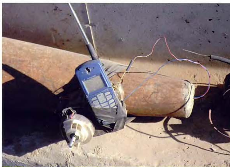
The insurgents' weapon of choice, circa 2004: a classic Baghdad IED, constructed with a South African 155-millimeter artillery round wired to a cordless phone, a nine-volt battery and a timer from a washing machine.
