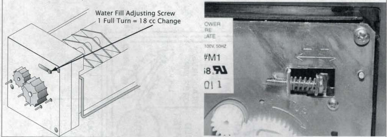
Figure 8-95 Water Fill Adjustment
