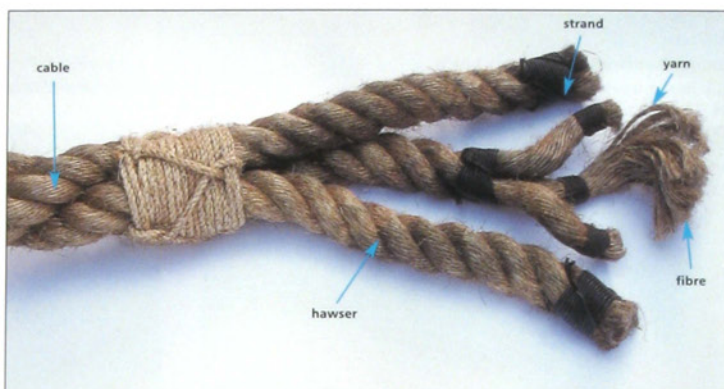
A lefthanded (or S-laid) cable consists of three righthanded (Z-laid) hawsers. Each of these ropes has three lefthanded (counterclockwise) strands made from numerous righthanded (clockwise) yarns, spun from vegetable fibres.
