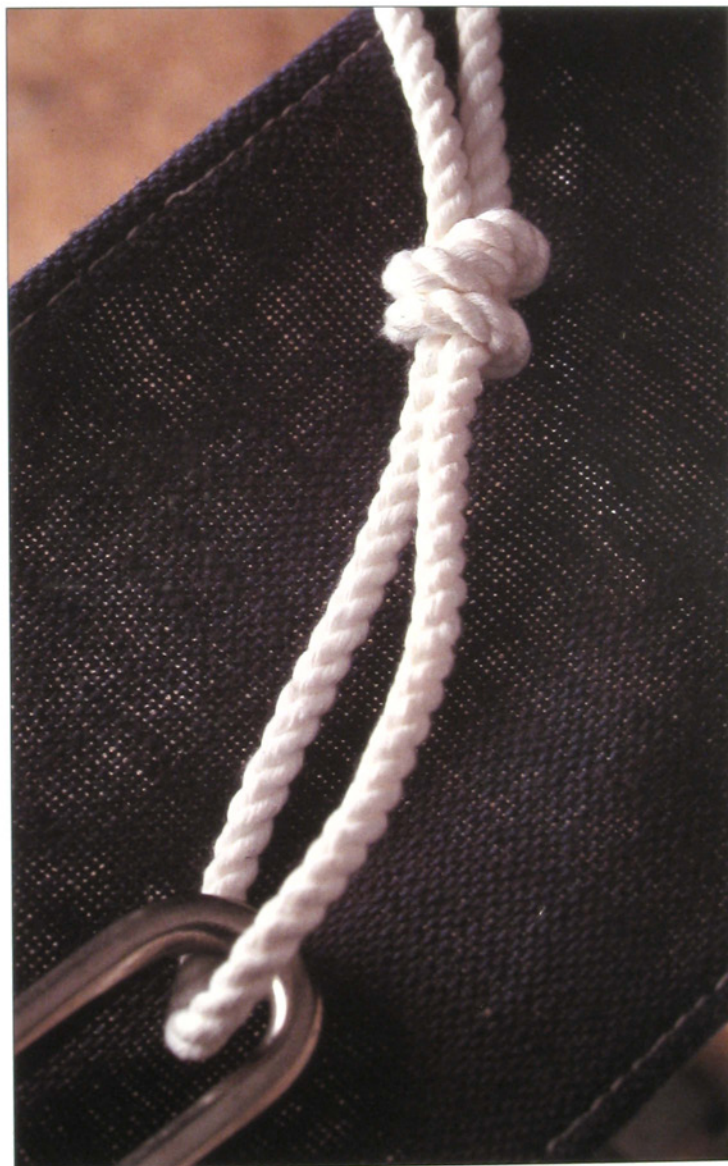
1 Tie the working end around the shackle.
