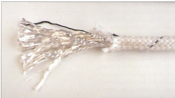
A 14 mm ( \frac{7}{12} in) diameter, soft matt polyester, 16-plait sheath encloses a hawser-laid core of several thousand high-tenacity polyester filaments.
