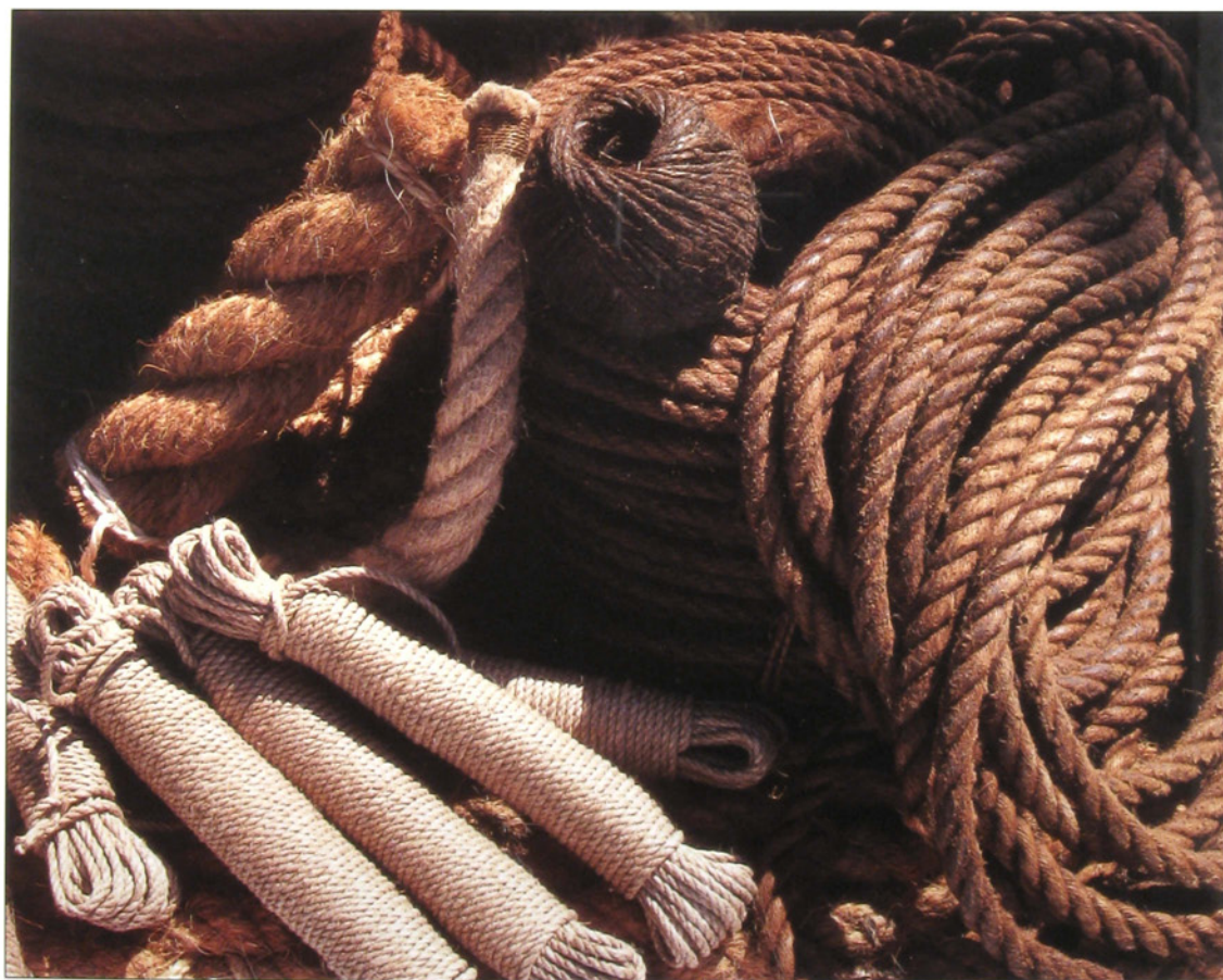
♦ BELOW Codline and water-resistant coir contrast with darkly tarred and weatherproofed, aromatic hemp hawsers and spun yarn.
