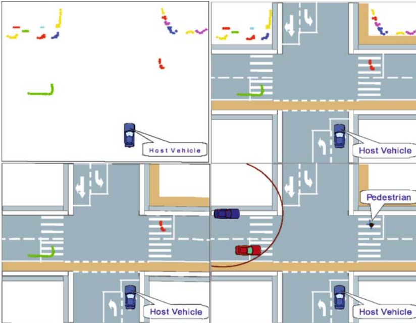
Fig. 3. Steps of the Cooperative Pre-Data-Fusion showing (a) a raw range profile, (b) map association, (c) tracked objects, and (d) cooperative VANET-data association.
