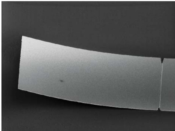
Fig. 1. SEM picture of the released tungsten-titanium cantilever on \text{SiO}_2 .
