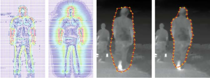
Fig. 2. Gradient vector field of a FIR pedestrian with bidirectional gradient direction and a decreasing gradient strength from red to blue. Gradient vector field with GVF after 0 (a, left) and 120 (d, right) iterations. Approximation of a pedestrian shape with an active contour model based on GVF after 8 (a) and finally in the stable stage after 24 (d) iterations.
