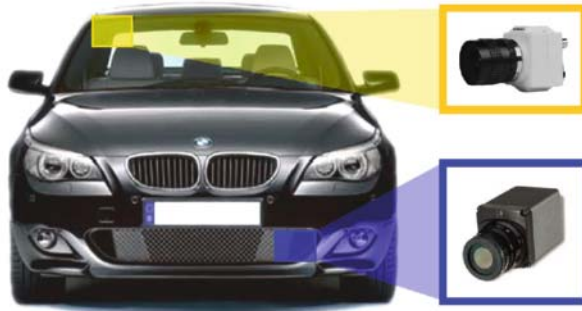
Fig. 5. Mounting locations of the video camera (top) and the far infrared image device (bottom) on the experimental car.
