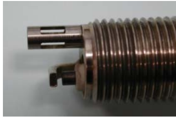
Fig. 3. Spark plug head with eccentrically placed ignition electrodes and absorption path
