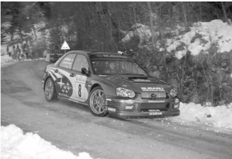
Fig. 7.35 Tommi Makinen hooks the front left wheel of his 2003 Subaru WRC off the tarmac and ensures a large yaw moment will be available shortly (courtesy of Prodrive)
