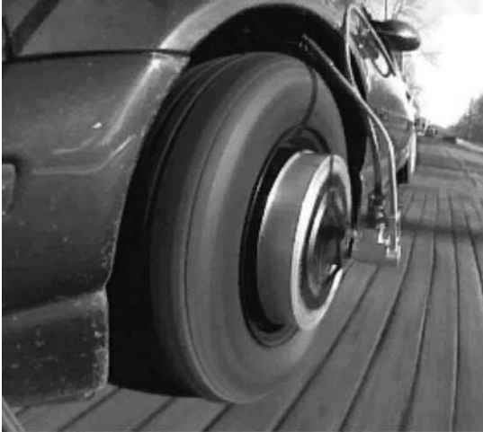
Fig. 5.62 Proving ground measurements at the wheel centre for durability analysis (provided courtesy of MSC.Software)
