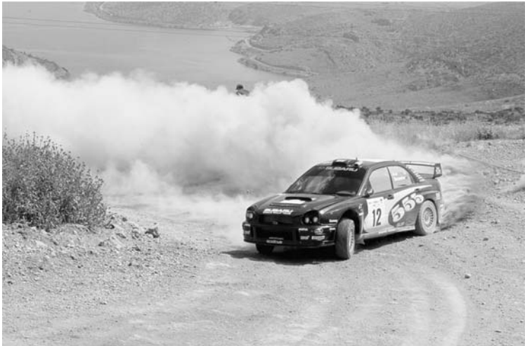
Fig. 6.47 Large body slip angles are unavailable to normal drivers except as part of an accident. Subaru WRC, Greece 2002 (courtesy of Prodrive)
