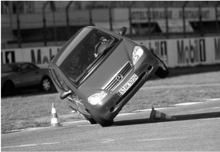
Fig. 1.1 Rollover of the Mercedes A-Class (courtesy of Auto Motor und Sport )
