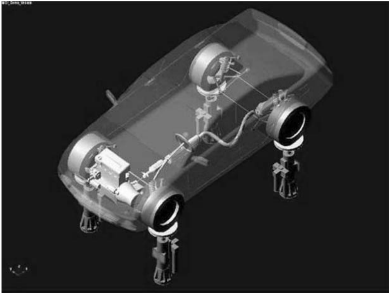
Fig. 6.2 A detailed multibody systems vehicle model (provided courtesy of MSC.Software)
