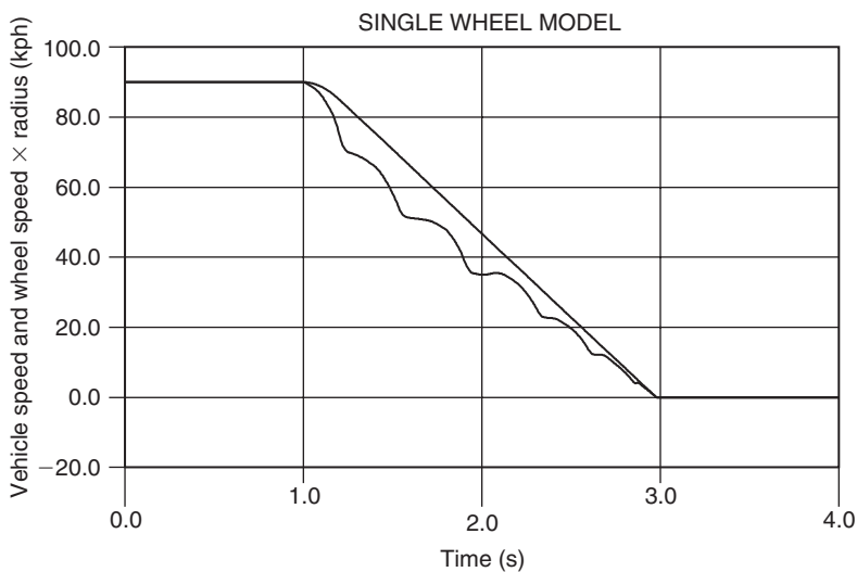
Fig. 6.32 Plot of vehicle speed and wheel speed during ABS braking simulation
