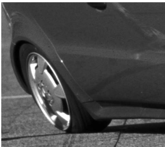
Fig. 5.1 An example of tyre deflection under hard cornering (courtesy of Auto Motor und Sport )
