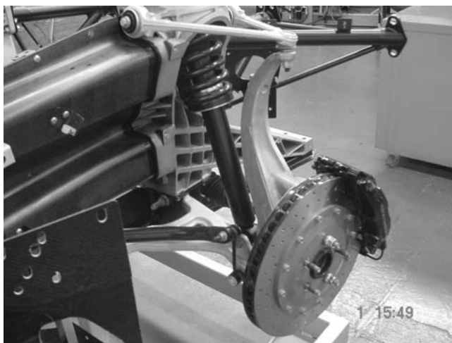
Fig. 4.1 Aston Martin Vanquish double wishbone front suspension system
