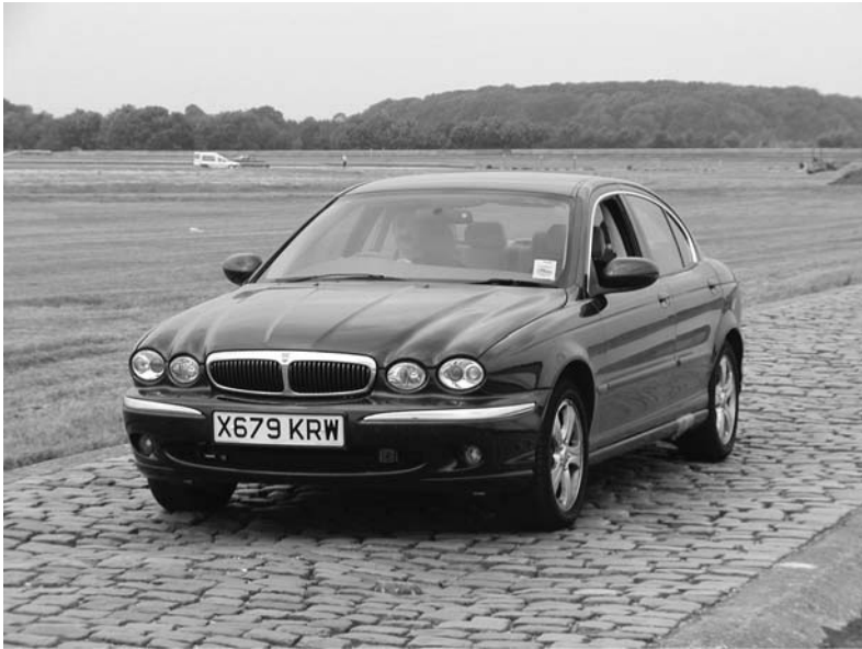
Fig. 4.44 Vehicle durability testing on cobbled road surface (provided courtesy of Jaguar Cars Ltd)
