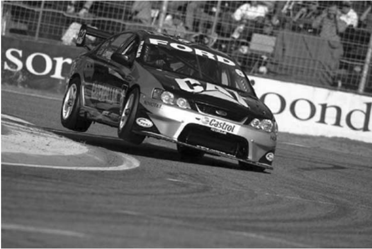
Fig. 4.10 The combination of anti-roll geometry to give a single 'roll centre' between left and right wheels is clearly nonsensical when the loading is strongly asymmetric – even when the asymmetry is less extreme than the racing Ford Falcon shown here.
