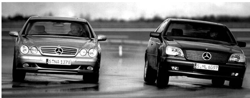
Fig. 8.2 Mercedes Active Body Control (ABC) in action at high lateral accelerations – around 1 degree of body roll (a combination of tyre compliance and some programmed roll compliance for ‘feel’) with the ABC car compared to 4.5 degrees of body roll for the passively suspended car (courtesy of Auto Motor und Sport )
