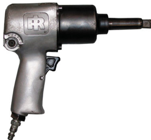
FIGURE 1-55 A typical 1/2-inch drive air impact wrench. The direction of rotation can be changed to loosen or tighten a fastener.
