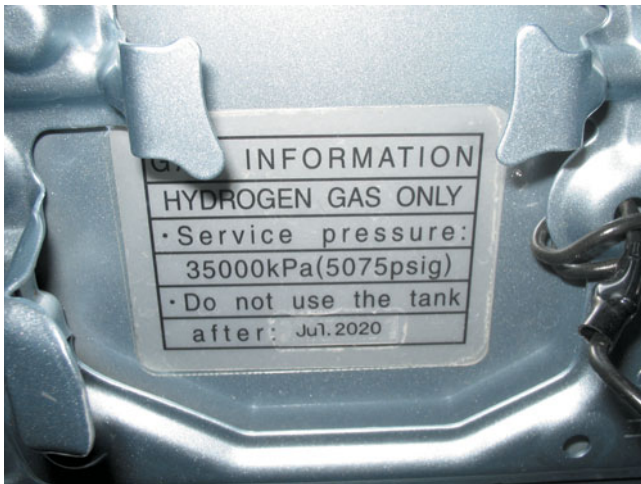
FIGURE 32-23 Note that high-pressure hydrogen storage tanks must be replaced in 2020.
