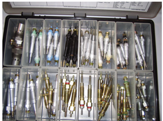
FIGURE 4-14 A glow plug assortment showing the various types and sizes of glow plugs used. Always use the specified glow plugs.
