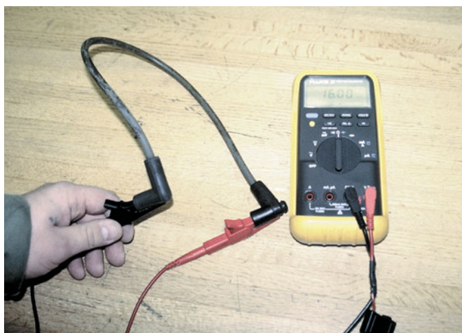
FIGURE 29-31 Measuring the resistance of a spark plug wire with a multimeter set to the ohms position. The reading of 16.03 kΩ (16,030 ohms) is okay because the wire is about 2 feet long. Maximum allowable resistance for a spark plug wire this long would be 20 kΩ (20,000 ohms).
