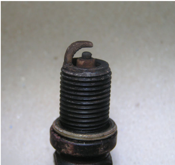
FIGURE 29-39 A worn spark plug showing fuel and/or oil deposits.
