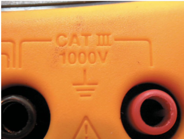
FIGURE 31-4 Be sure to only use a meter that is CAT III rated when taking electrical voltage measurements on a hybrid electric or electric vehicle.
