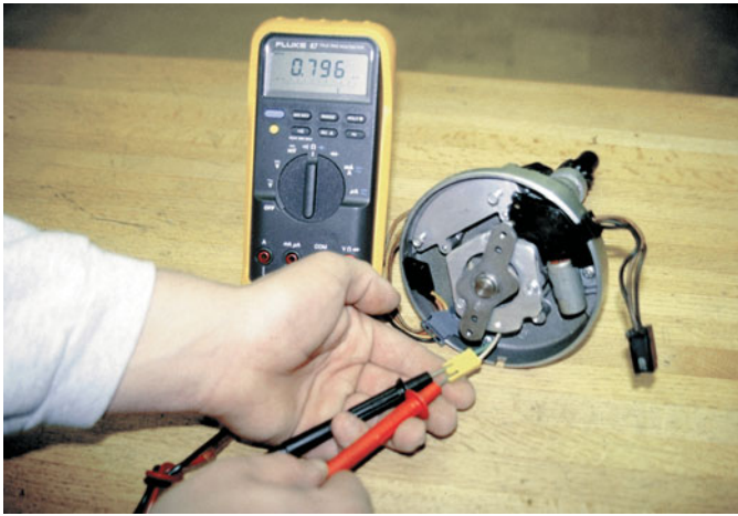
FIGURE 29-25 Measuring the resistance of an HEI pickup coil using a digital multimeter set to the ohms position. The reading on the face of the meter is 0.796 kΩ, or 796 ohms in the middle of the 500- to 1,500-ohm specifications.
