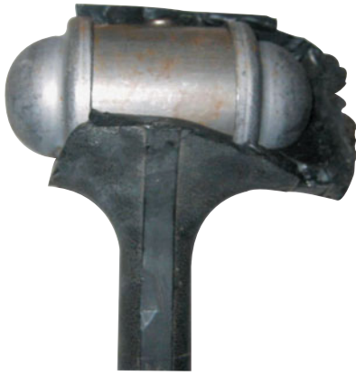
FIGURE 1-35 A dead-blow hammer that was left outside in freezing weather. The plastic covering was damaged, which destroyed this hammer. The lead shot is encased in the metal housing and then covered.
