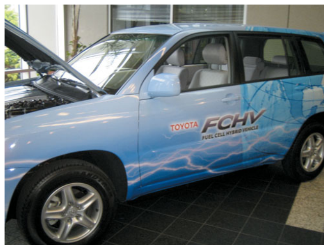
FIGURE 32-4 The Toyota FCHV is based on the Highlander platform and uses much of Toyota's Hybrid Synergy Drive (HSD) technology in its design.
