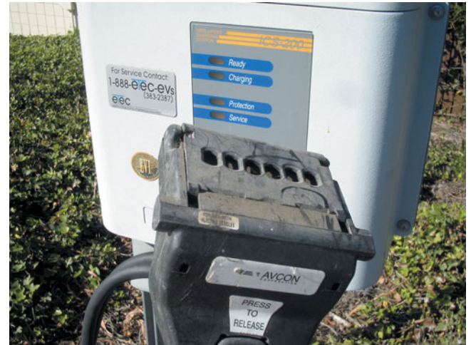
FIGURE 32-29 A conductive-type charging connector. This type of battery charging connector is sometimes called an AVCON connector, named for the manufacturer.
