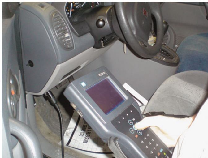
FIGURE 30-17 The first step in the reprogramming procedure is to determine the current software installed using a scan tool. Not all scan tools can be used. In most cases using the factory scan tool is needed for reprogramming unless the scan tool is equipped to handle reprogramming.
