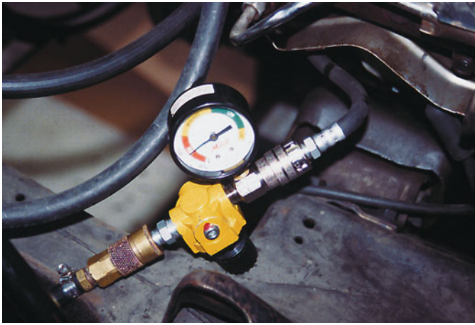
FIGURE 10-13 A typical handheld cylinder leakage tester.
