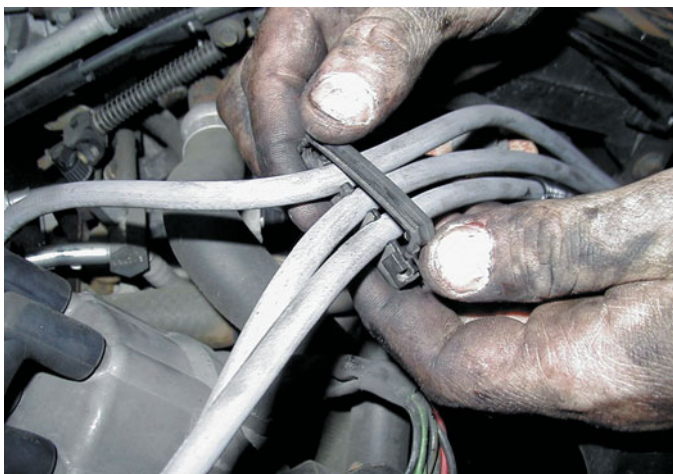
FIGURE 29-33 Always take the time to install spark plug wires back into the original holding brackets (wiring combs).
