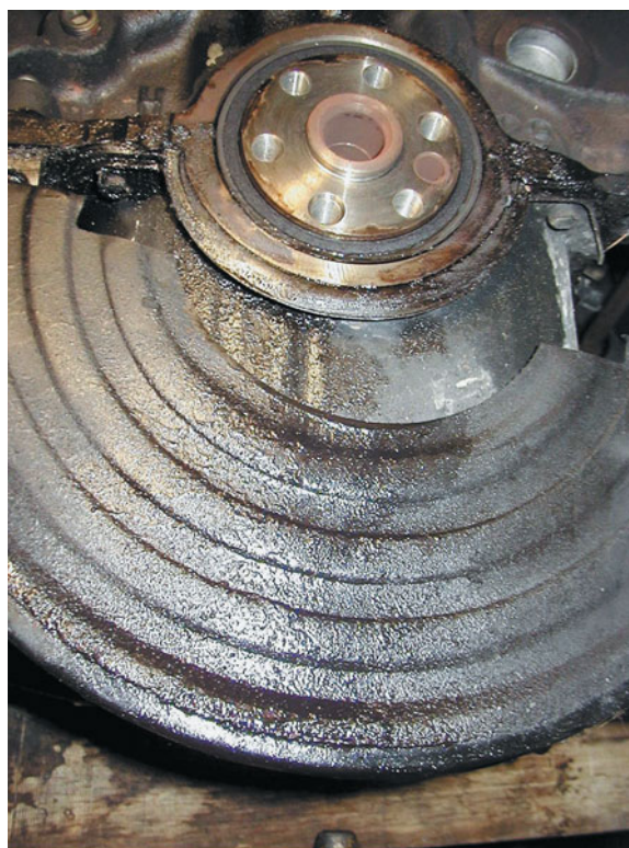
FIGURE 10-4 The transmission and flexplate (flywheel) were removed to check the exact location of this oil leak. The rear main seal and/or the oil pan gasket could be the cause of this leak.
