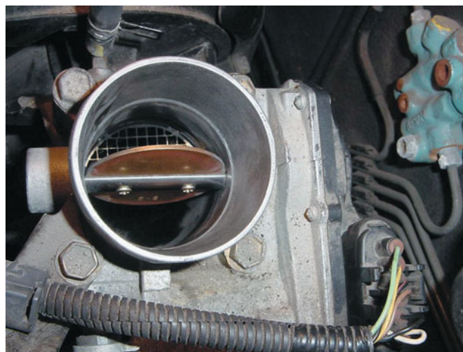
FIGURE 22-11 The throttle plate stayed where it was moved by the technician, which indicates that there is a problem with the electronic throttle body control assembly.
