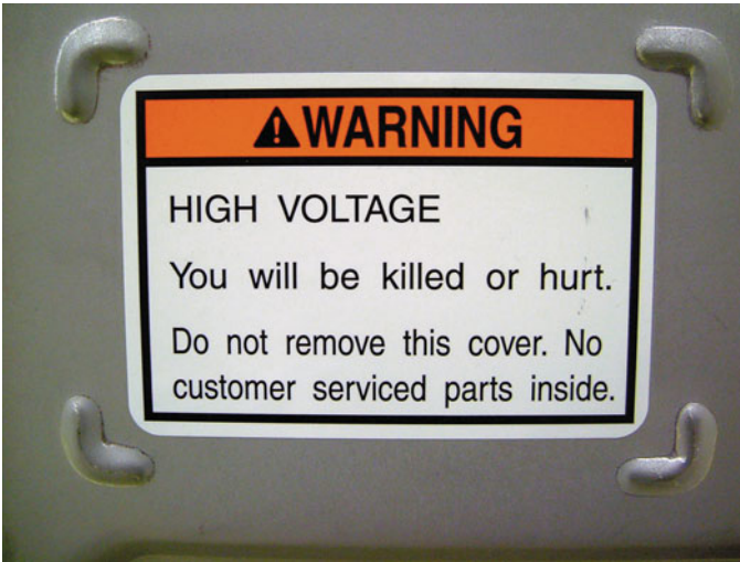
FIGURE 1-84 A warning label on a Honda hybrid warns that a person can be killed because of the high-voltage circuits under the cover.
