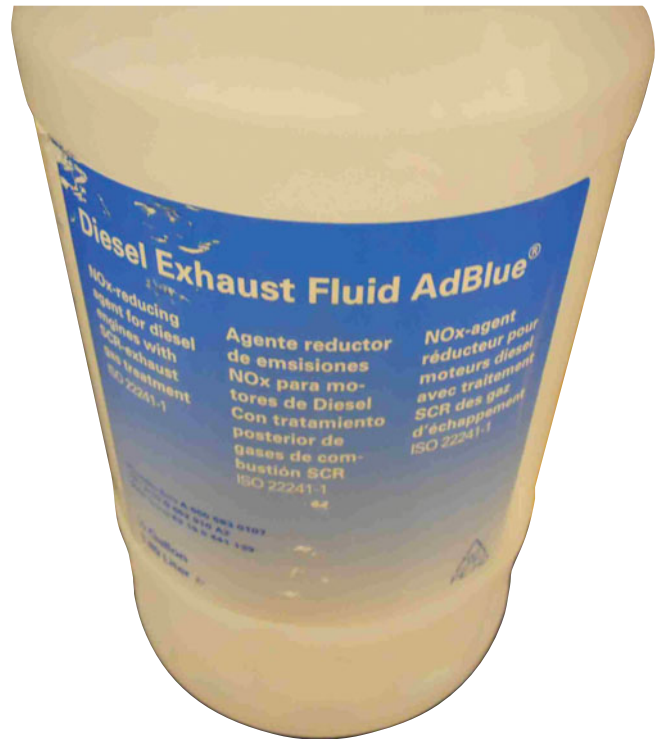
FIGURE 4-30 Diesel exhaust fluid cost $3 to $4 a gallon and is housed in a separate container that holds from 5 to 10 gallons, or enough to last until the next scheduled oil change in most diesel vehicles that use SCR.
