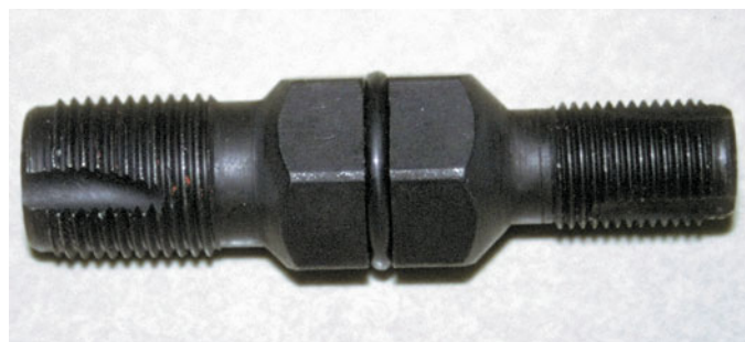
FIGURE 29-37 A spark plug thread chaser is a low-cost tool that hopefully will not be used often but is necessary to use to clean the threads before new spark plugs are installed.
