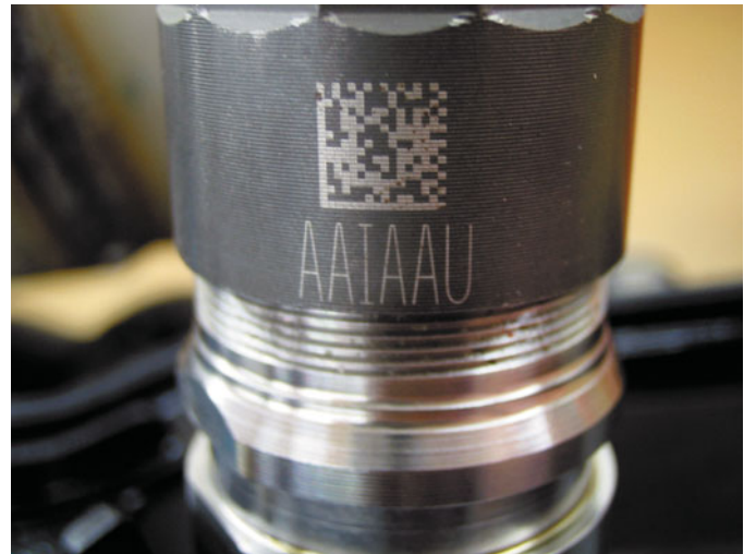
FIGURE 4-35 The letters on the side of this injector on a Cummins 6.7 liter diesel indicate the calibration number for the injector.
