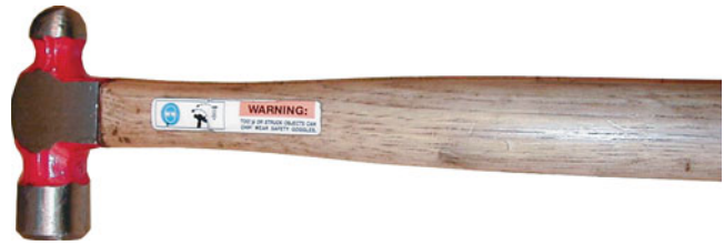
FIGURE 1-33 A typical ball-peen hammer.
