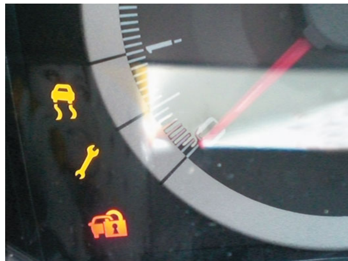
FIGURE 22-9 A wrench symbol warning lamp on a Ford vehicle. The symbol can also be green.
