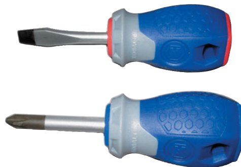
FIGURE 1-30 Two stubby screwdrivers that are used to access screws that have limited space above. A straight blade is on top and a #2 Phillips screwdriver is on the bottom.
