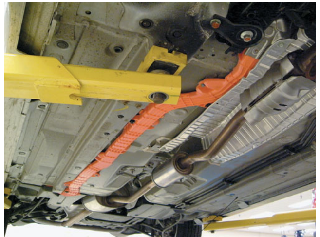
FIGURE 31-12 The high-voltage wiring on this Honda hybrid is colored orange for easy identification.
