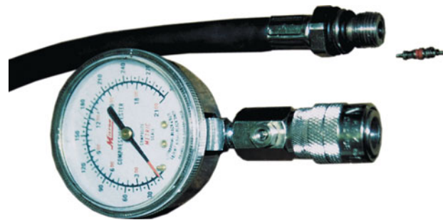
FIGURE 10-10 A two-piece compression gauge set. The threaded hose is screwed into the spark plug hole after removing the spark plug. The gauge part is then snapped onto the end of the hose.
