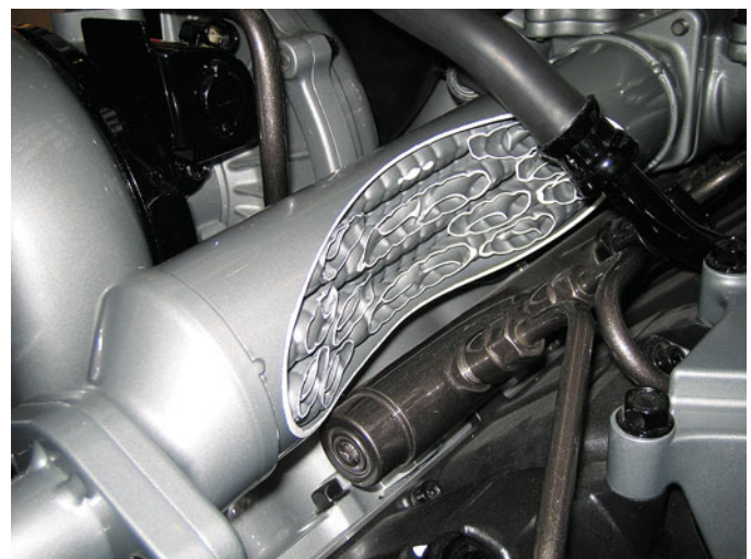
FIGURE 4-21 A cutaway showing the exhaust cooler. The cooler the exhaust is, the more effective it is in controlling \text{NO}_x emissions.
