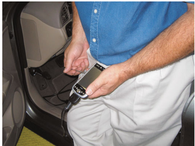
FIGURE 30-12 Some scan tools use pocket PCs, which make it very convenient to use.
