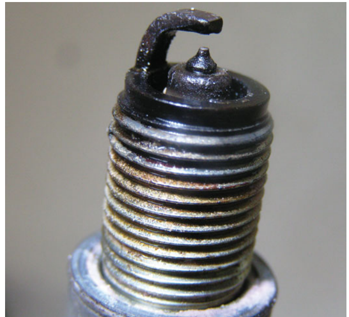
FIGURE 29-41 A platinum tipped spark plug that is fuel soaked indicating a fault with the fuel system or the ignition system causing the spark plug to not fire.
