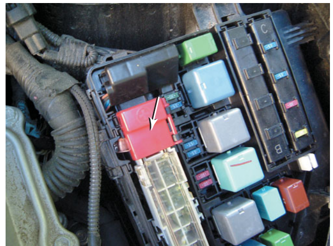
FIGURE 31-8 The underhood 12-volt jump-start terminal on this 2004+ Toyota Prius has a red plastic cover with a “+” sign. The positive booster cable clamp will attach directly to the vertical metal bracket.
