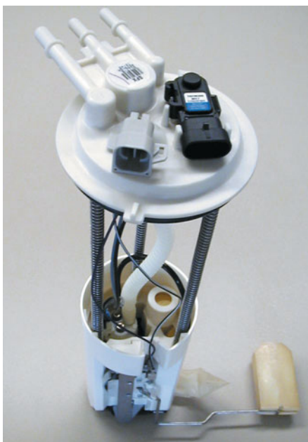
FIGURE 19-16 A typical fuel pump module assembly, which includes the pickup strainer and fuel pump, as well as the fuel-pressure sensor and fuel level sensing unit.
