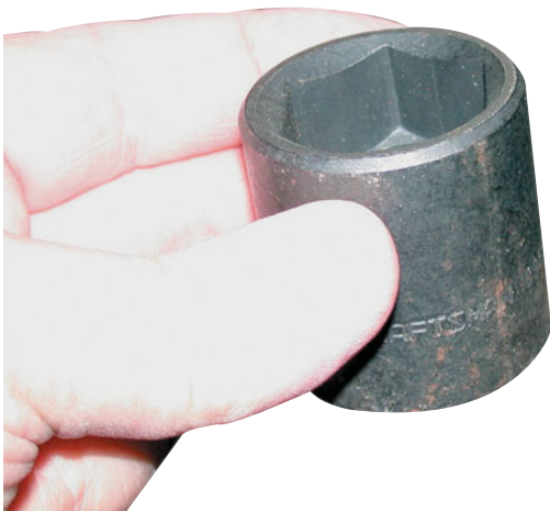
FIGURE 1-57 A black impact socket. Always use an impact-type socket whenever using an impact wrench to avoid the possibility of shattering the socket, which could cause personal injury.
