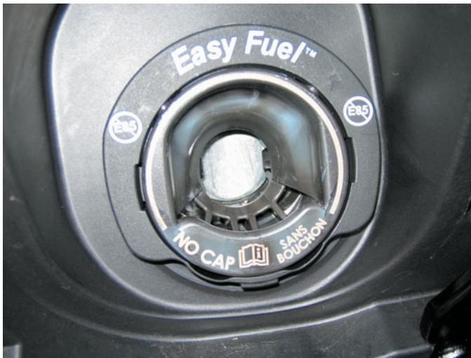
FIGURE 25-1 A capless system from a Ford Flex does not use a replaceable cap; instead, it is spring-loaded closed.
