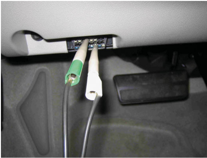
FIGURE 12-28 Use front-probe terminals to access the data link connector. Always follow the specified back-probe and front-probe procedures as found in service information.
