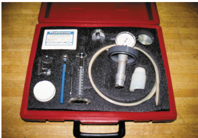
FIGURE 5-2 A gasoline testing kit, including an insulated container where water at 100°F is used to heat a container holding a small sample of gasoline. The reading on the pressure gauge is the Reid vapor pressure (RVP).
