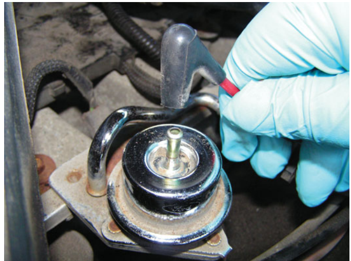
FIGURE 23-1 If the vacuum hose is removed from the fuel-pressure regulator when the engine is running, the fuel pressure should increase. If it does not increase, then the fuel pump is not capable of supplying adequate pressure or the fuel-pressure regulator is defective. If gasoline is visible in the vacuum hose, the regulator is leaking and should be replaced.
