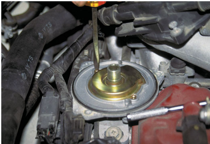
FIGURE 29-11 A light shield is being installed on an optical distributor before the rotor is attached.
