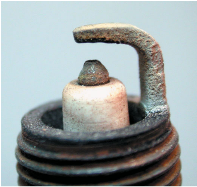
FIGURE 29-38 A normally worn spark plug that uses a tapered platinum-tipped center electrode.
