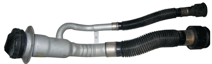
FIGURE 19-4 Vehicles equipped with onboard refueling vapor recovery usually have a reduced-size fill tube.
