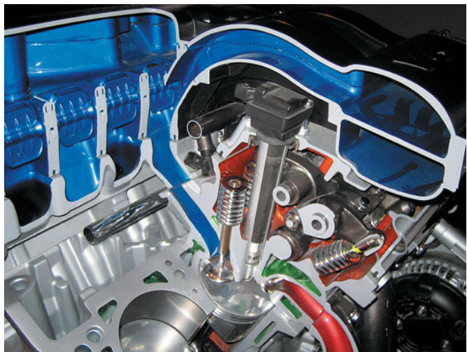
FIGURE 8-11 The air flowing into the engine can be directed through long or short runners for best performance and fuel economy.
