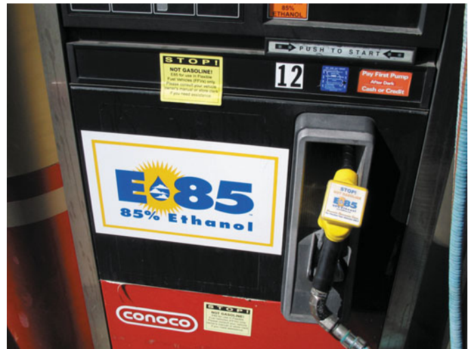
FIGURE 6-5 A pump for E85 (85% ethanol and 15% gasoline). E85 is available in more locations every year.
