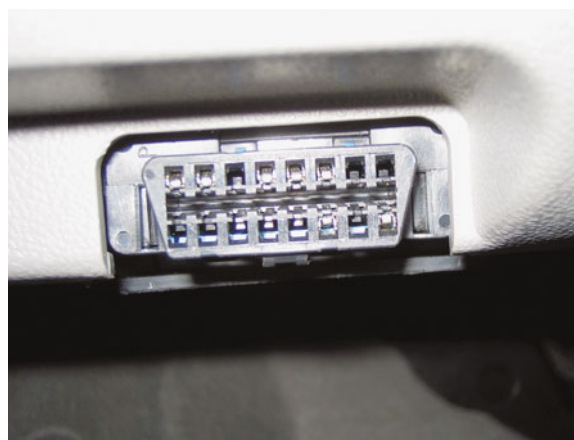
FIGURE 30-16 A typical OBD-II data link connector (DLC). The location varies with make and model and may even be covered, but a tool is not needed to gain access. Check service information for the exact location if needed.
