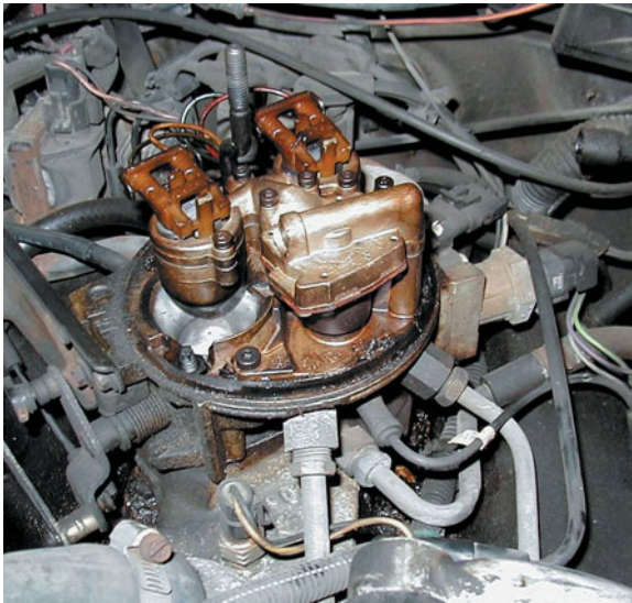
FIGURE 8-7 A throttle-body injection (TBI) unit used on a GM V-6 engine.
