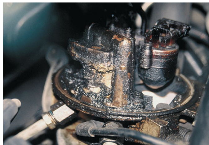
FIGURE 23-3 A clogged PCV system caused the engine oil fumes to be drawn into the air cleaner assembly. This is what the technician discovered during a visual inspection.
