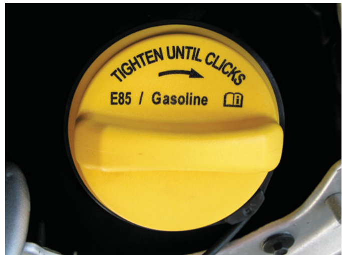
FIGURE 6-6 A flex-fuel vehicle often has a yellow gas cap, which is labeled E85/gasoline.
