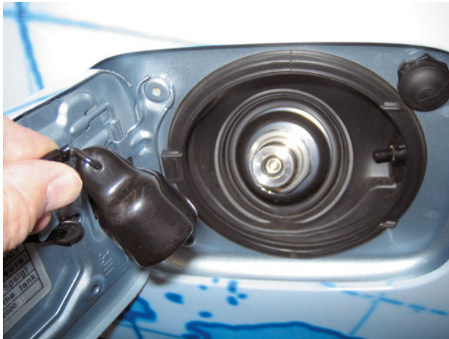
FIGURE 32-22 The high-pressure fitting used to refuel a fuel-cell hybrid vehicle.
