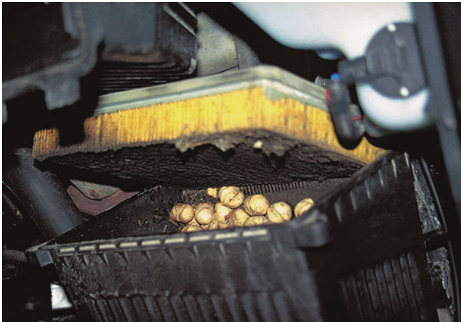
FIGURE 30-4 This is what was found when removing an air filter from a vehicle that had a lack-of-power concern. Obviously the nuts were deposited by squirrels or some other animal, blocking a lot of the airflow into the engine.
