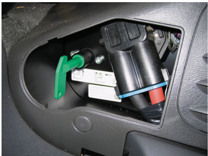
FIGURE 1-87 The shutoff switch on a GM parallel hybrid truck is green because this system uses 42 volts instead of higher, possibly fatal voltages used in other hybrid vehicles.
