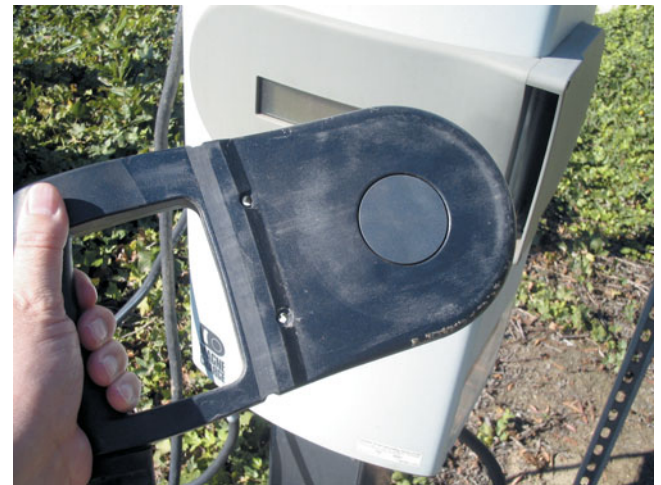
FIGURE 32-30 An inductive-type electric vehicle battery charger connector. This type of connector fits into a charging slot in the vehicle but does not make electrical contact.
