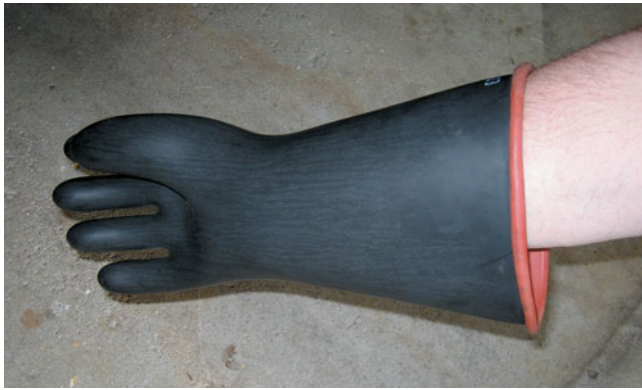
FIGURE 31-1 Rubber lineman's gloves protect the wearer from a shock hazard.
