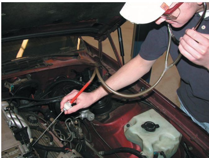
FIGURE 23-4 All fuel injectors should make the same sound with the engine running at idle speed. A lack of sound indicates a possible electrically open injector or a break in the wiring. A defective computer could also be the cause of a lack of clicking (pulsing) of the injectors.
