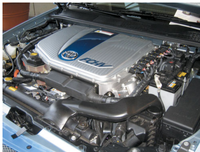
FIGURE 32-11 Space is limited at the front of the Toyota FCHV engine compartment, so an auxiliary heat exchanger is located under the vehicle to help cool the fuel-cell stack.
