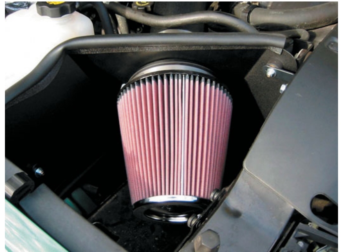
FIGURE 8-22 A high-performance aftermarket air filter often can increase airflow into the engine for more power.
