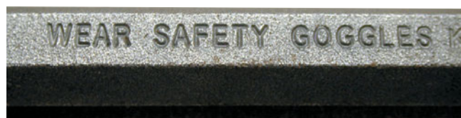
FIGURE 1-47 Warning stamped on the side of a punch warning that goggles should be worn when using this tool. Always follow safety warnings.
