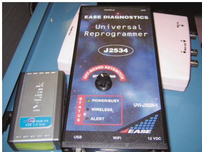
FIGURE 30-22 A typical J2534 universal reprogrammer that uses the J2534 standards.
