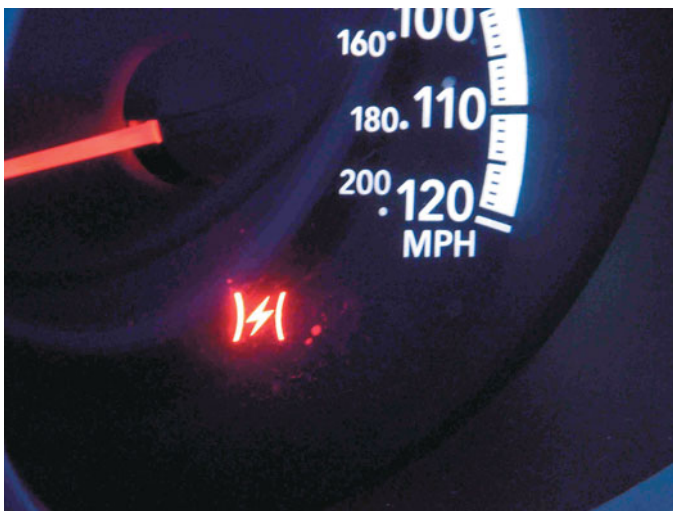
FIGURE 22-10 A symbol used on a Chrysler vehicle indicating a fault with the electronic throttle control (ETC).
