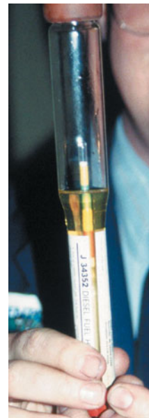
FIGURE 7-2 Testing the API viscosity of a diesel fuel sample using a hydrometer.
