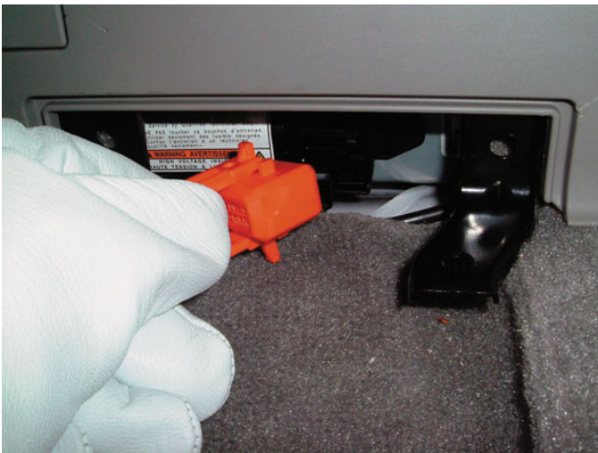
FIGURE 1-85 The high-voltage disconnect switch is in the trunk area on a Toyota Prius. Insulated rubber lineman's gloves should be worn when removing this plug. (Courtesy of Tony Martin)
