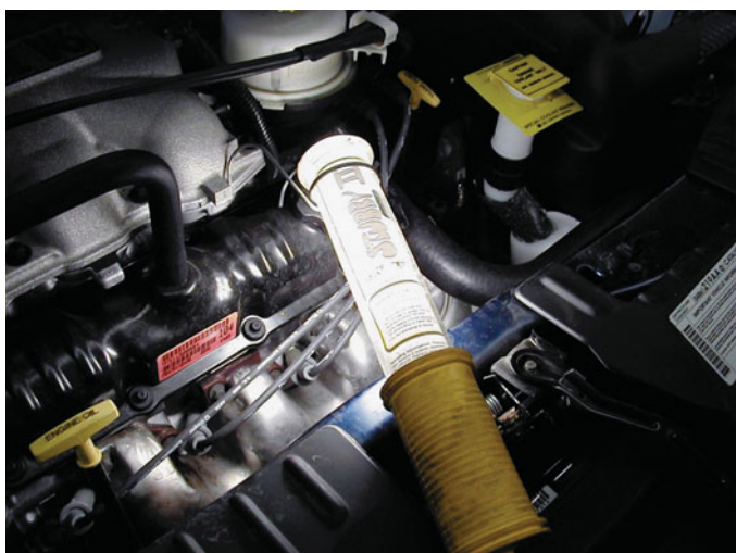
FIGURE 1-54 A fluorescent trouble light operates cooler and is safer to use in the shop because it is protected against accidental breakage where gasoline or other flammable liquids would happen to come in contact with the light.
