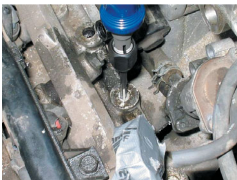
FIGURE 26-11 Removing the EGR passage plugs from the intake manifold on a Honda.
