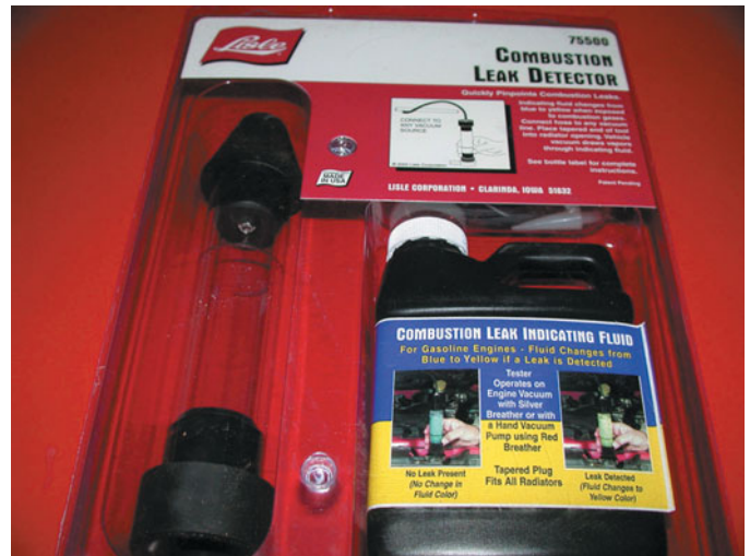
FIGURE 10-28 A tester that uses a blue liquid to check for exhaust gases in the exhaust, which would indicate a head gasket leak problem.
