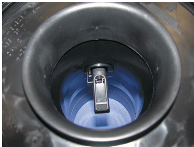
FIGURE 16-4 The sensing wire in a typical hot wire mass airflow sensor.
