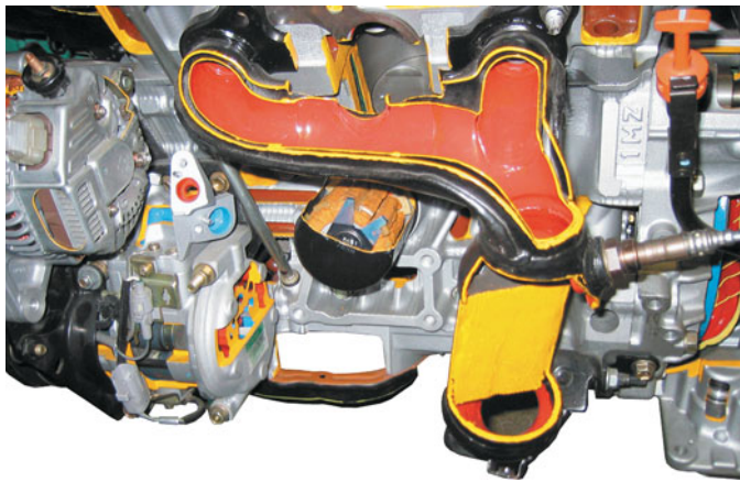
FIGURE 8-15 This exhaust manifold (red area) is equipped with a heat shield to help retain heat and reduce exhaust emissions.
