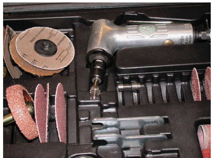
FIGURE 1-59 This typical die grinder surface preparation kit includes the air-operated die grinder as well as a variety of sanding disks for smoothing surfaces or removing rust.
