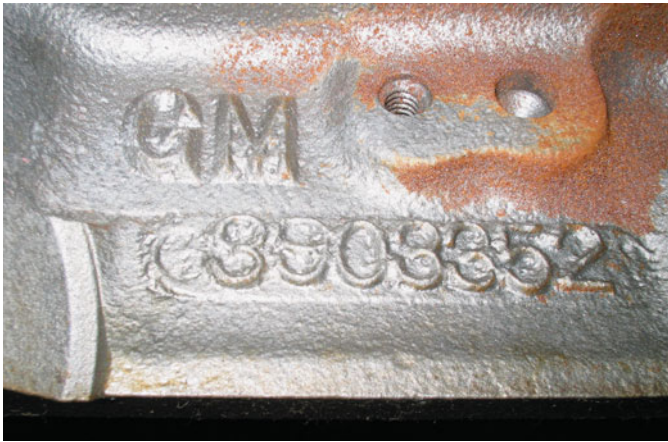
FIGURE 1-4 Casting numbers on major components can be either cast or stamped.
