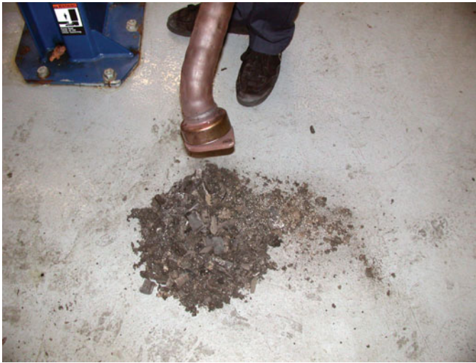
FIGURE 28-8 A catalytic converter that rattles when tapped was removed, and the substrate, or what was left of it, fell out. This converter has to be replaced and the root cause of why it failed found and corrected.
