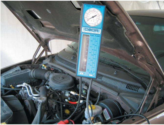
FIGURE 19-27 A fuel system tester connected in series in the fuel system so all of the fuel used flows through the meter, which displays the rate flow and the fuel pressure.
