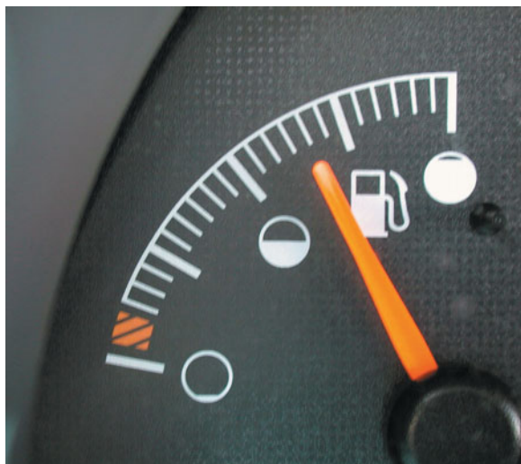
FIGURE 25-16 The fuel level must be above 15% and below 85% before the EVAP monitor will run on most vehicles.
