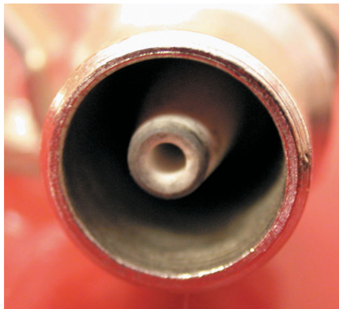
FIGURE 29-23 A close-up showing the recessed center electrode on a spark tester. It is recessed 3/8 inch into the shell, and the spark must then jump another 3/8 inch to the shell for a total gap of 3/4 inch.
