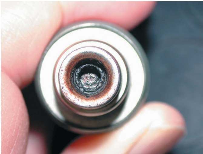
FIGURE 23-14 If an injector has the specified resistance, this does not mean that it is okay. This injector had the specified resistance, yet it did not deliver the correct amount of fuel because it was clogged.
