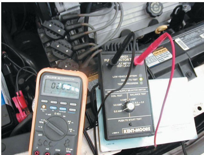
FIGURE 23-16 An injector tester being used to check the voltage drop through the injector while the tester is sending current through the injectors. This test is used to check the coil inside the injector. This same tester can be used to check for equal pressure drop of each injector by pulsing the injector on for 500 ms.
