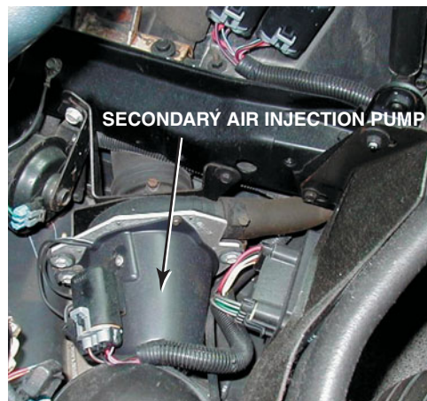
FIGURE 27-11 A typical electric motor-driven SAI pump. This unit is on a Chevrolet Corvette and only works when the engine is cold.
