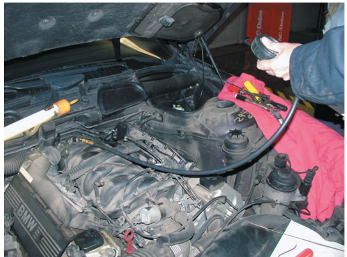
FIGURE 23-7 Checking the fuel pressure using a fuel-pressure gauge connected to the Schrader valve.
