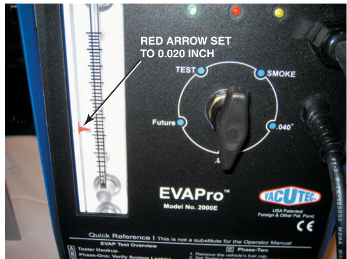
FIGURE 25-9 To test for a leak, this tester was set to the 0.020-inch hole and turned on. The ball rose in the scale on the left, and the red arrow was moved to that location. If when testing the system for leaks the ball rises higher than the arrow, then the leak is larger than 0.02 inch. If the ball does not rise to the level of the arrow, the leak is smaller than 0.020 inch.
