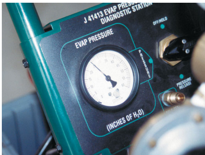
FIGURE 25-11 An emission tester that uses nitrogen to pressurize the fuel system.
