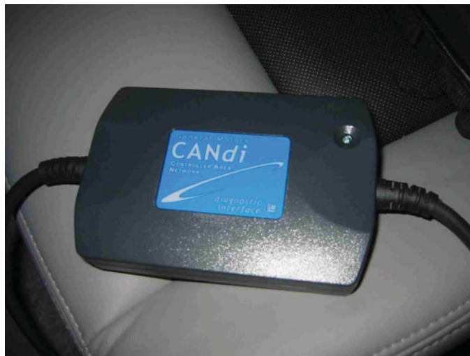
FIGURE 12-12 A CANdi module will flash the green LED rapidly if communication is detected.
