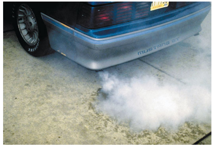
FIGURE 10-2 White steam is usually an indication of a blown (defective) cylinder head gasket that allows engine coolant to flow into the combustion chamber where it is turned to steam.
