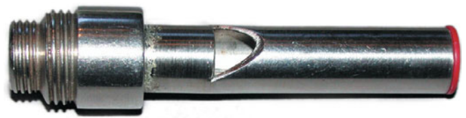
FIGURE 10-14 A whistle stop used to find top dead center. Remove the spark plug and install the whistle stop, then rotate the engine by hand. When the whistle stops making a sound, the piston is at the top.
