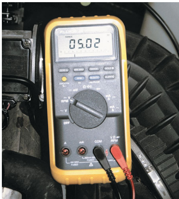
FIGURE 14-5 Checking the 5-volt reference from the computer being applied to the TP sensor with the ignition switch on (engine off). The reading for this vehicle (5.02 volts DC) is within the normal range for the reference voltage of 4.9 to 5.1 volts.
