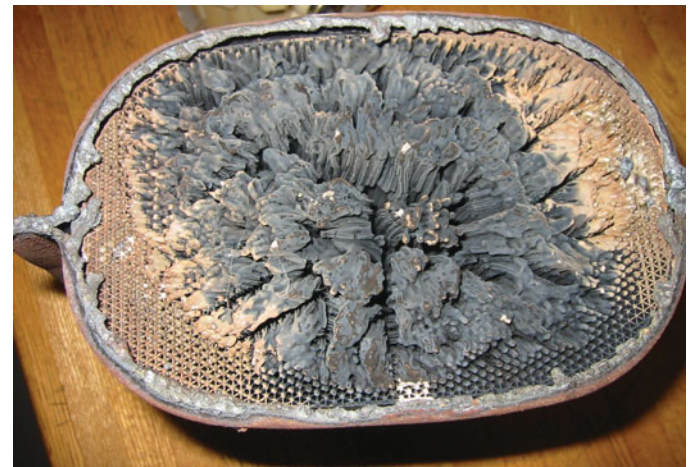
FIGURE 28-10 This partially melted catalytic converter tested okay at idle but had excessive back pressure at idle speeds.
