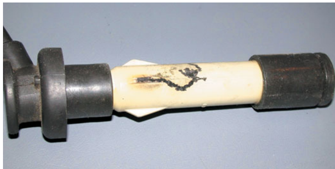
FIGURE 29-30 This spark plug boot on an overhead camshaft engine has been arcing to the valve cover causing a misfire to occur.
