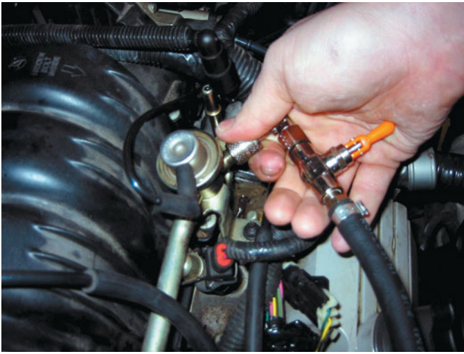
FIGURE 19-22 The Schrader valve on this General Motors 3800 V-6 is located next to the fuel-pressure regulator.
