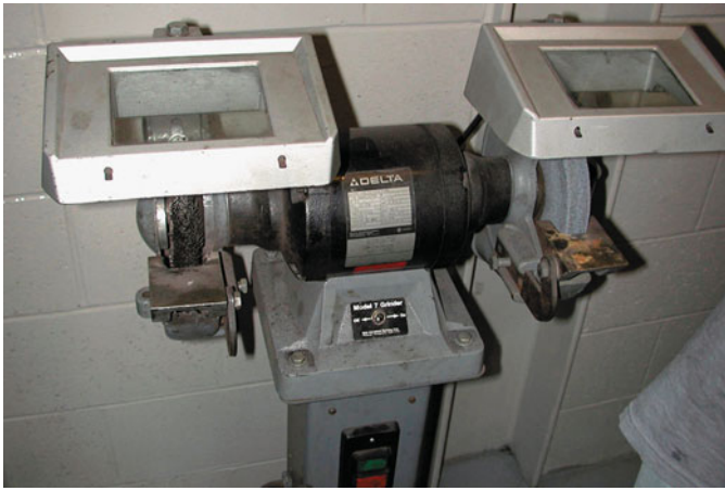
FIGURE 1-60 A typical pedestal grinder with a wire wheel on the left side and a stone wheel on the right side. Even though this machine is equipped with guards, safety glasses or a face shield should always be worn whenever using a grinder or wire wheel.
