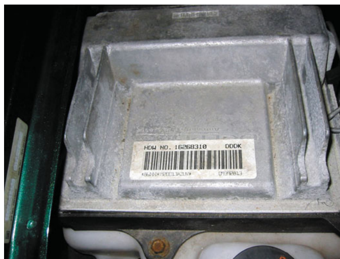
FIGURE 1-3 A typical calibration code sticker on the case of a controller. The information on the sticker is often needed when ordering parts or a replacement controller.
