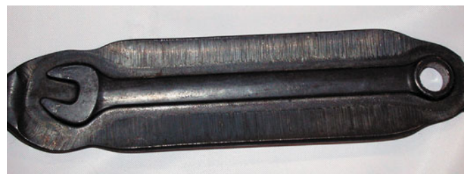
FIGURE 1-15 A forged wrench after it has been forged but before the flashing, which is the extra material around the wrench, has been removed.
