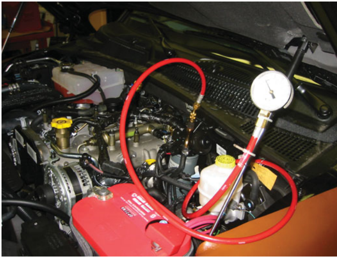
FIGURE 4-32 A pressure gauge checking the fuel pressure from the lift pump on a Cummins 6.7 liter diesel.
