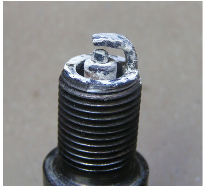
FIGURE 29-40 A spark plug from an engine that had a blown head gasket. The white deposits could be from the aluminum of the piston or from the additives in the coolant.
