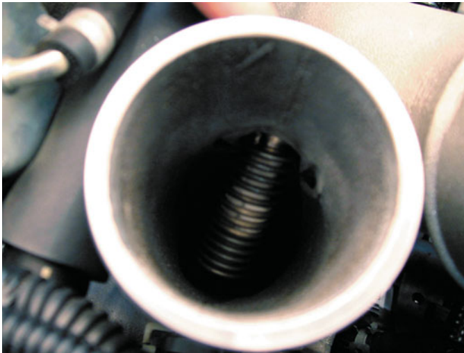
FIGURE 4-16 A wire-wound electric heater is used to warm the intake air on some diesel engines.
