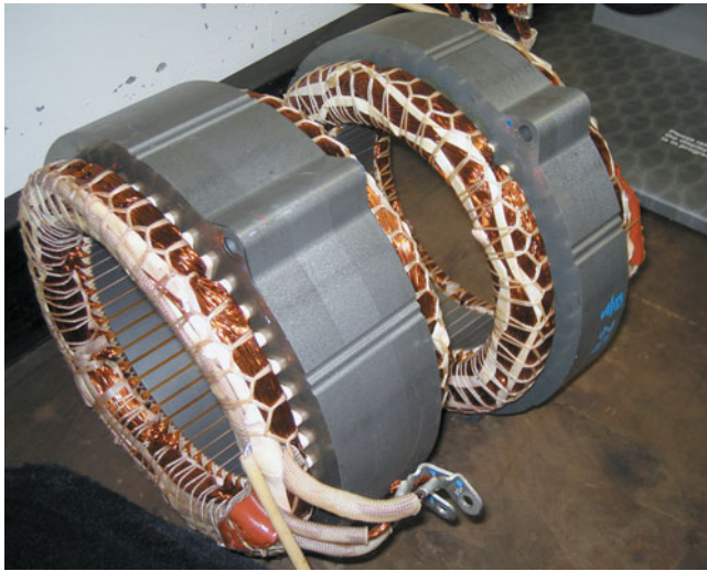
FIGURE 32-15 Drive motors in fuel-cell hybrid vehicles often use stator assemblies similar to ones found in Toyota hybrid electric vehicles. The rotor turns inside the stator and has permanent magnets on its outer circumference.
