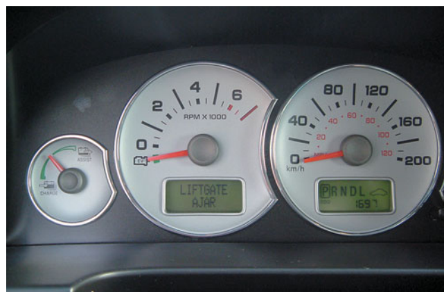
FIGURE 31-6 The Ford Escape Hybrid instrument panel showing the vehicle in park and the tachometer on “EV” instead of 0 RPM. This means that the gasoline engine could start at any time depending on the state-of-charge of the high-voltage batteries and other factors.
