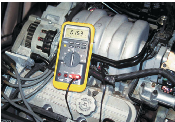
FIGURE 23-12 To measure fuel-injector resistance, a technician constructed a short wiring harness with a double banana plug that fits into the V and COM terminals of the meter and an injector connector at the other end. This setup makes checking resistance of fuel injectors quick and easy.
