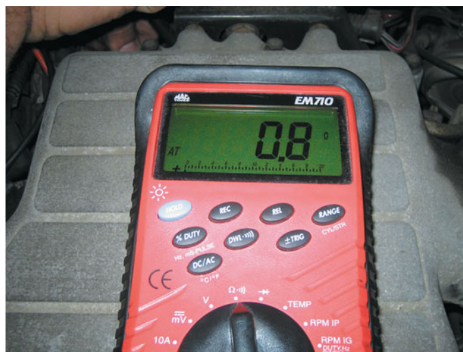
FIGURE 23-13 (a) The meter is connected to read one group of three 12-ohm injectors. The result should be 4 ohms, and this reading is a little low, indicating that at least one injector is shorted (low resistance). (b) This meter is connected to the other group of three injectors and indicates that most, if not all three, injectors are shorted. The technician replaced all six injectors, and the engine ran great.
