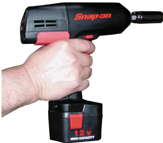
FIGURE 1-56 A typical battery-powered 3/8-inch drive impact wrench.
