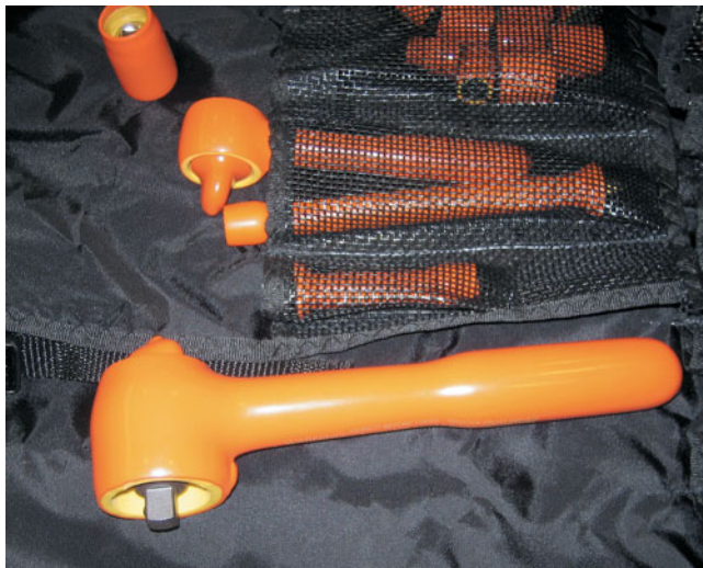
FIGURE 31-11 Insulated tools, such as this socket set, would provide an additional margin of safety to the service technician when working around high-voltage components and systems.
