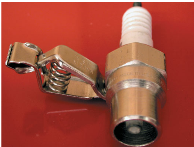
FIGURE 29-22 A spark tester looks like a regular spark plug with an alligator clip attached to the shell. This tester has a specified gap that requires at least 25,000 volts (25 kV) to fire.
