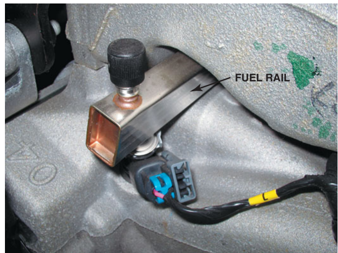
FIGURE 20-15 A rectangular-shaped fuel rail is used to help dampen fuel system pulsations and noise caused by the injectors opening and closing.
