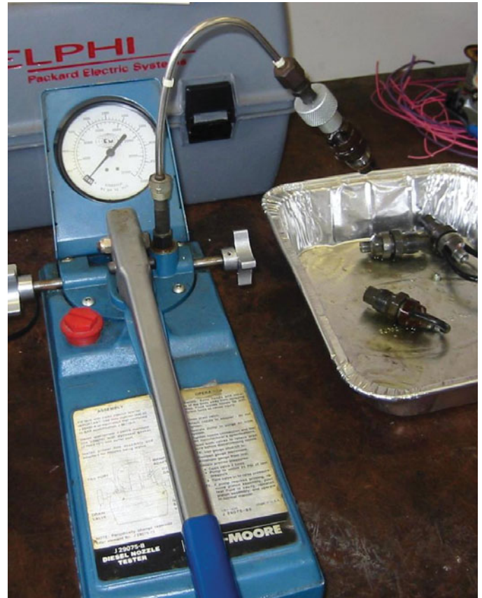
FIGURE 4-34 A typical pop tester used to check the spray pattern of a diesel engine injector.
