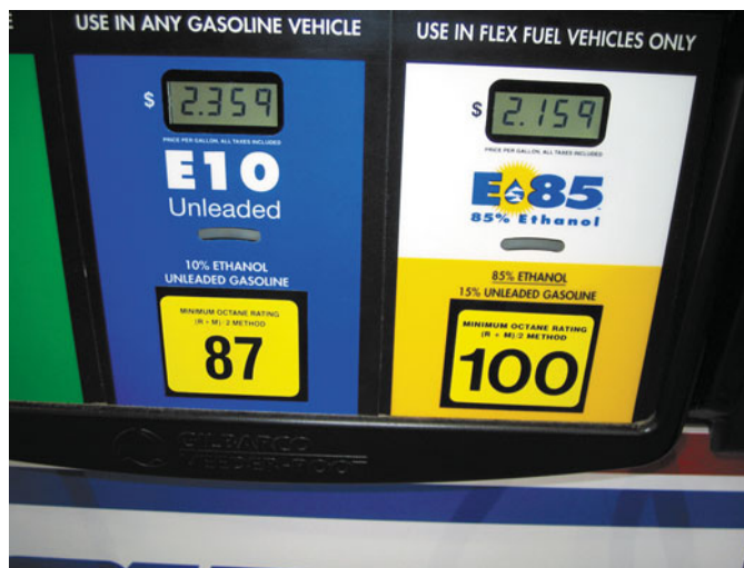
FIGURE 5-10 This refueling pump indicates that the gasoline is blended with 10% ethanol (ethyl alcohol) and can be used in any gasoline vehicle. E85 contains 85% ethanol and can be used only in vehicles specifically designed to use it.
