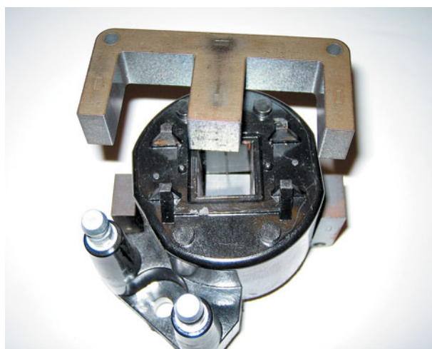
FIGURE 29-3 The steel lamination used in an E coil helps increase the magnetic field strength, which helps the coil produce higher energy output for a more complete combustion in the cylinders.
