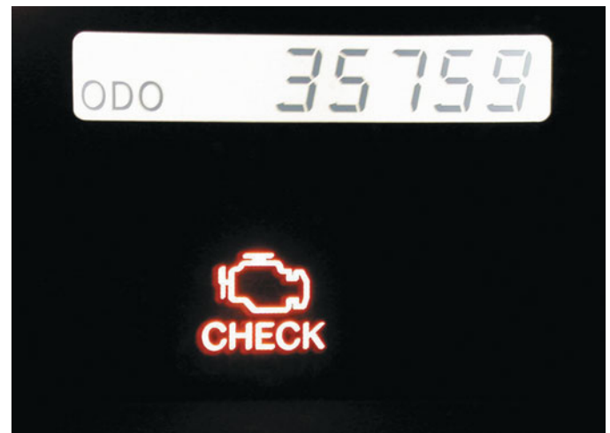
FIGURE 11-1 A typical malfunction indicator lamp (MIL) often labeled “check engine” or “service engine soon” (SES).
