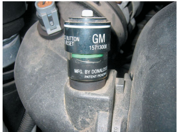
FIGURE 8-4 A typical air filter restriction indicator used on a General Motors truck engine. The indicator turns red when it detects enough restriction to require a filter replacement.
