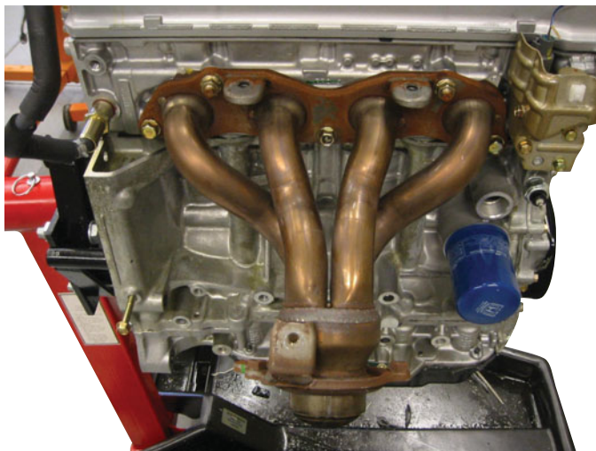
FIGURE 8-16 Many exhaust manifolds are constructed of steel tubing and are free flowing to improve engine performance.
