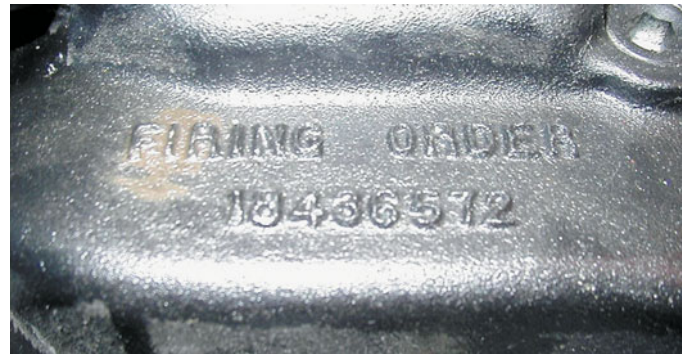
FIGURE 29-12 The firing order is cast or stamped on the intake manifold on most engines that have a distributor ignition.
