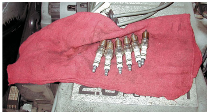
FIGURE 29-36 When removing spark plugs, it is wise to arrange them in the order by the cylinder they were removed from so that they can be compared and any problem can be identified with a particular cylinder.
