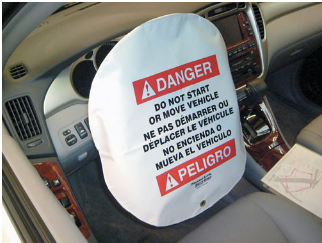
FIGURE 31-9 Using a warning cover over the steering wheel helps others realize that work is being performed on the high-voltage system and that no one is to attempt to start or move the vehicle.
