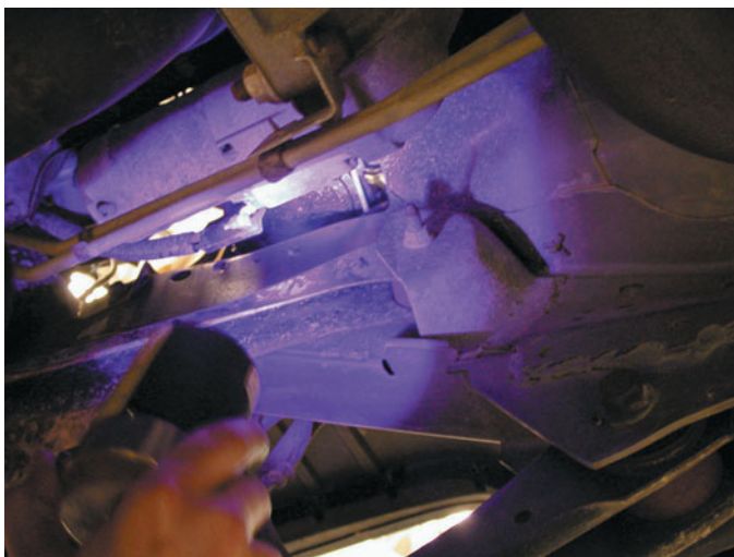
FIGURE 10-5 Using a black light to spot leaks after adding dye to the oil.
