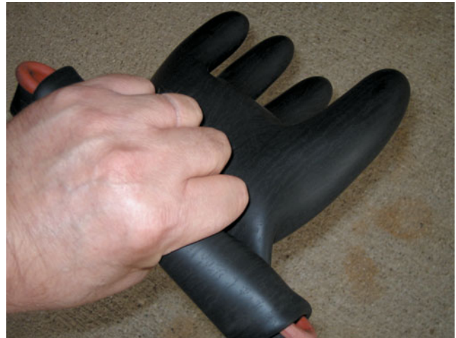
FIGURE 31-3 Checking rubber lineman's gloves for pinhole leaks.
