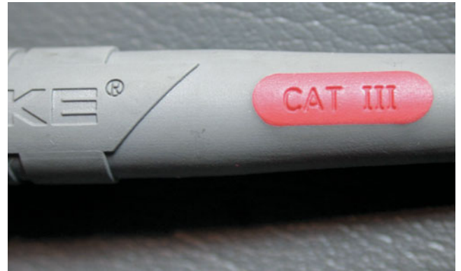
FIGURE 31-5 The meter leads should also be CAT III rated when checking voltages on a hybrid electric vehicle.
