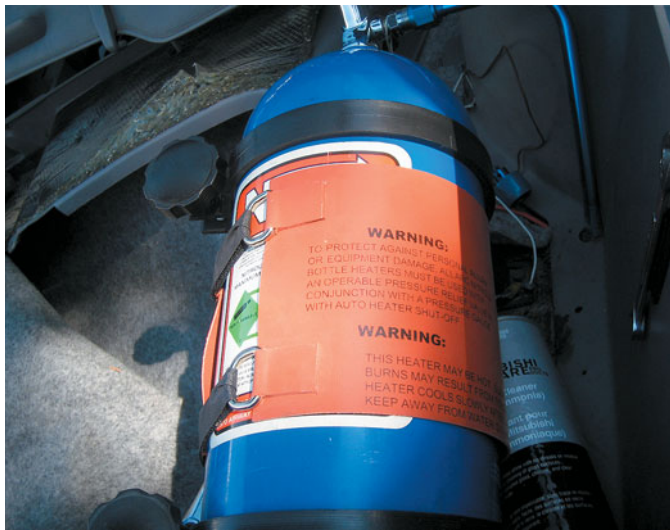
FIGURE 9-17 An electrical heating mat is installed on the bottle of nitrous oxide to increase the pressure of the gas inside.
