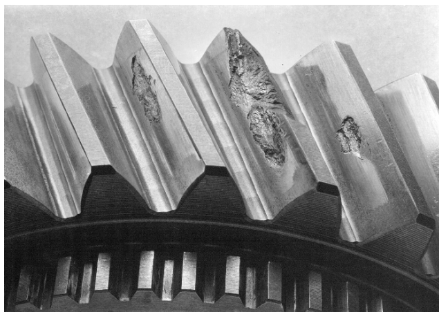
Fig. 7.4. Macropitting with tip fracture due to flank surface fatigue [7.40]
