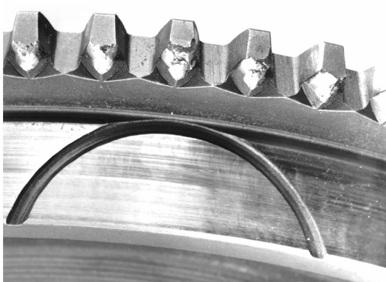
Fig. 9.16. Damage to the dogs of the selector teeth caused by grating. Ring groove in the friction cone of the commercial vehicle synchronizer hub
