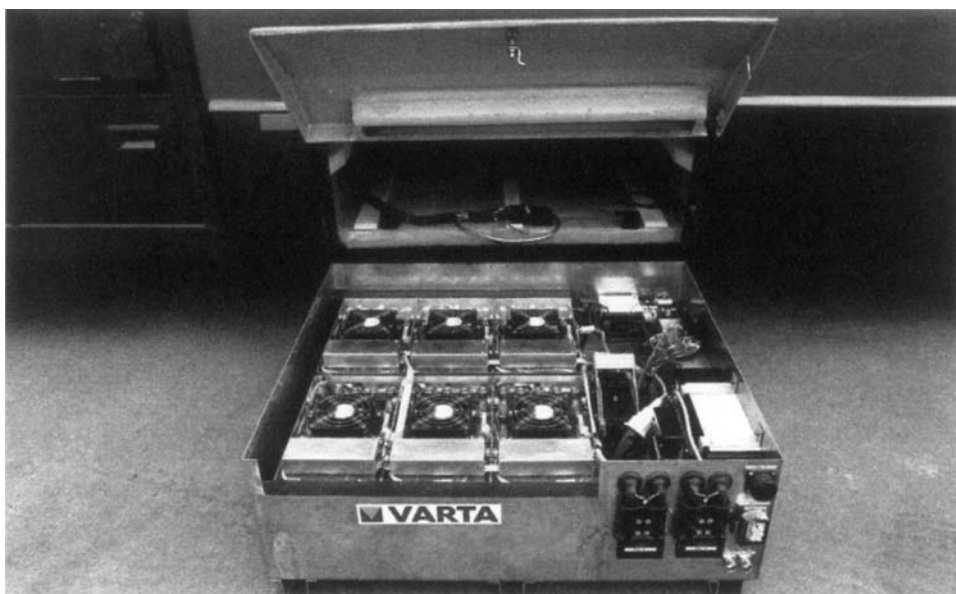
Figure 4.13 Cross-section of battery with nickel/metal hydride monoblocs.
