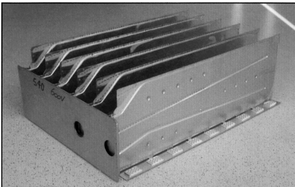
Figure 10.9 Z5C battery cooling plates.
