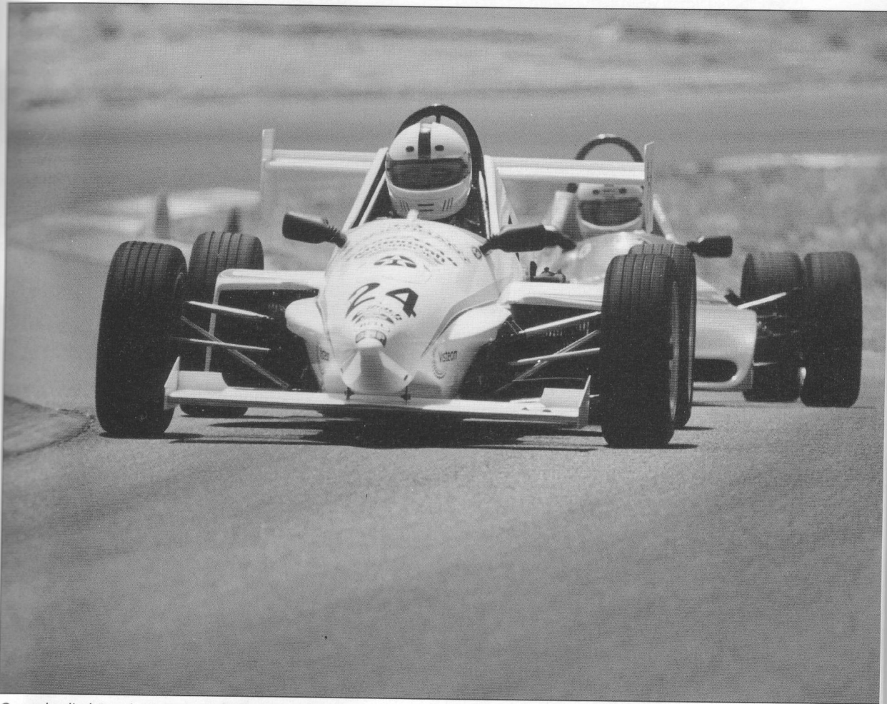
Our rebodied Bondurant Formula Ford featuring a new "F-1-Style" design with functional front and rear wings. Rick Scuteri
