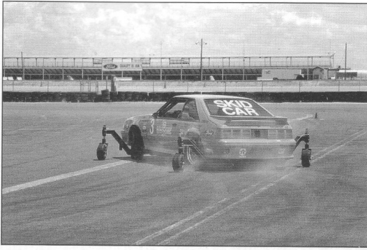
The Bondurant Skid Car in action, teaching students the principles of oversteer and understeer. Rick Scuteri
