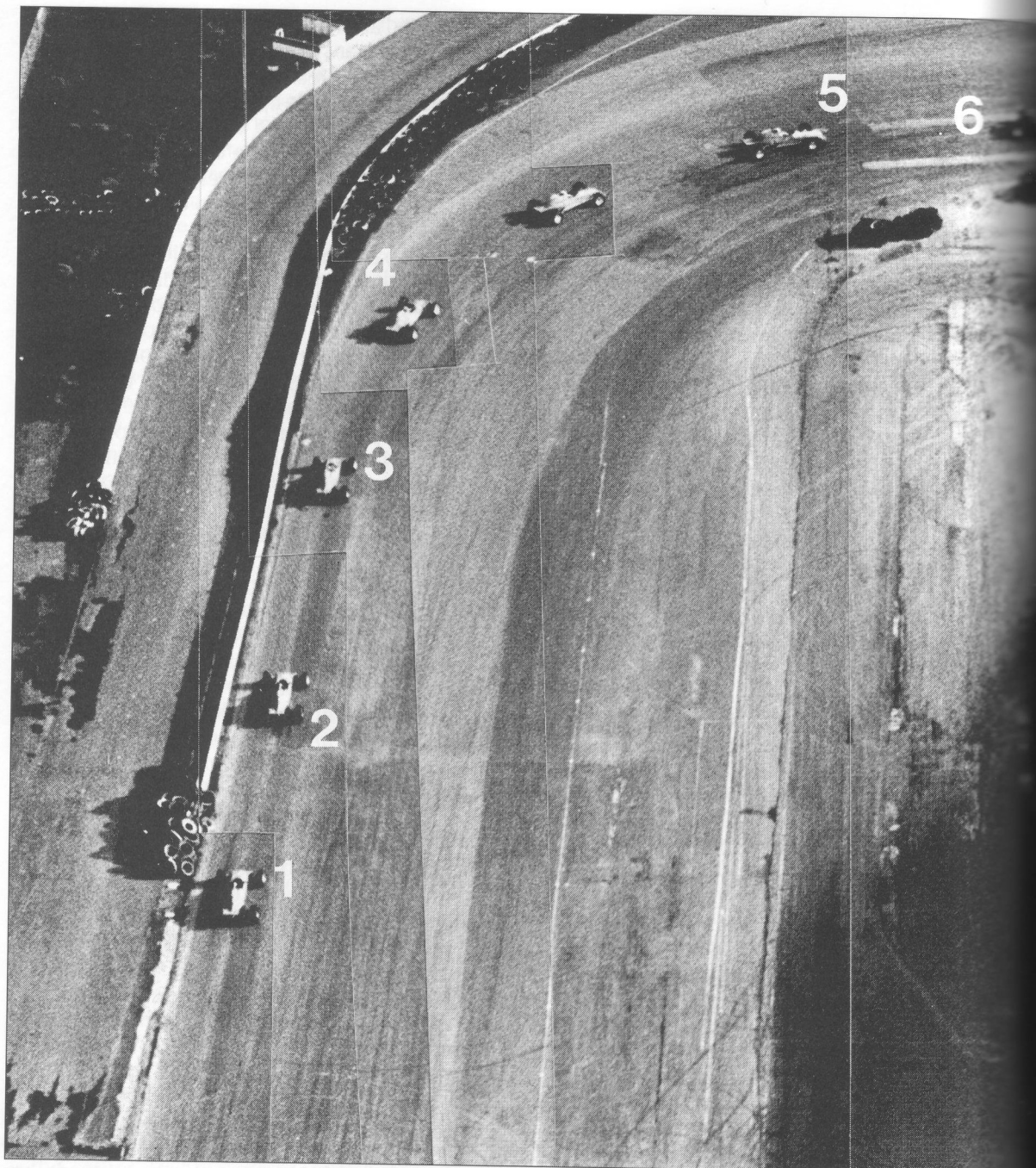
A composite of a corner. The numbers on the photo indicate the following actions: 1: Under full braking. 2: Start heel-and-toe downshift. 3: Complete downshift. 4: Start trail-braking. 5: Complete trail-braking. 6: Begin acceleration. 7: Under full acceleration. 8: Exit point. 9-10: This is the apex area. To put all of this in perspective, this section lasts approximately six to seven seconds in a Formula Ford.
