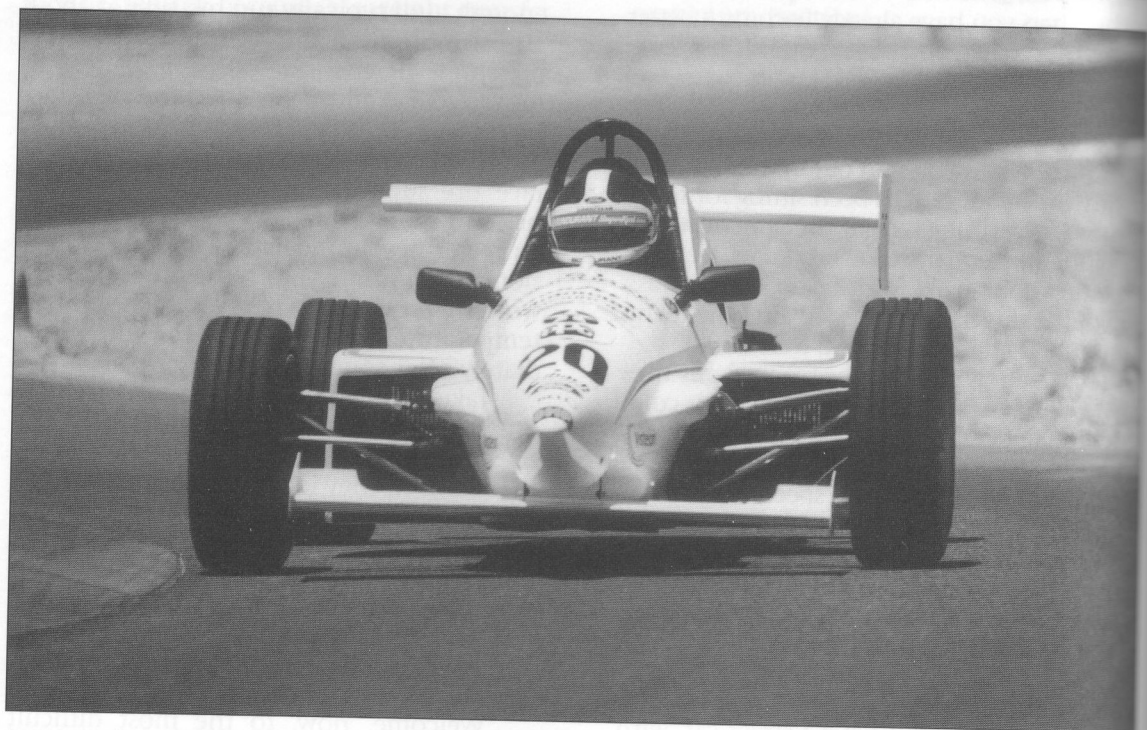
Entering a late-apex area. The car is stable but in a four-wheel drift under full acceleration. All four tire patches are working at their limits. Rick Scuteri
