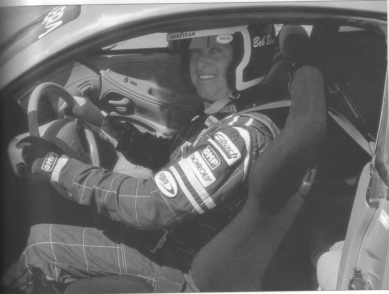
Proper seating position. Notice the upright position of the seat and the position of my arms and legs in relation to the steering wheel. Rick Scuteri
