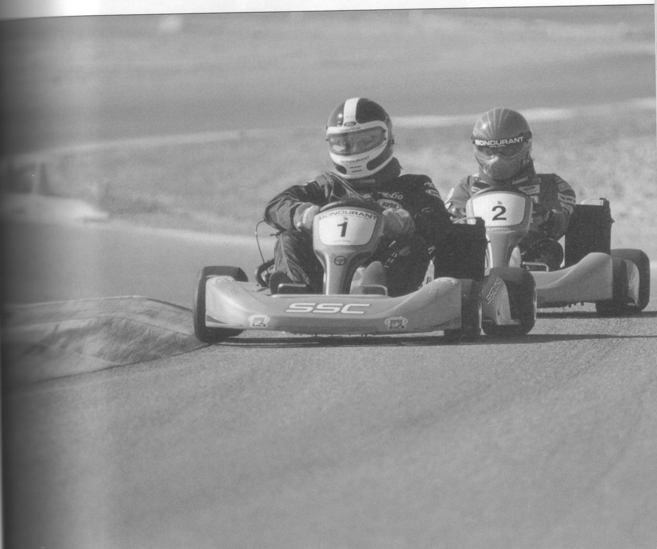
Bob Bondurant and Bryant Stodola in the heat of battle. The CRG Italian Shifter School Kart is powered by a Kawasaki 125-cc engine with a six-speed sequential gearbox. Rick Scuteri
