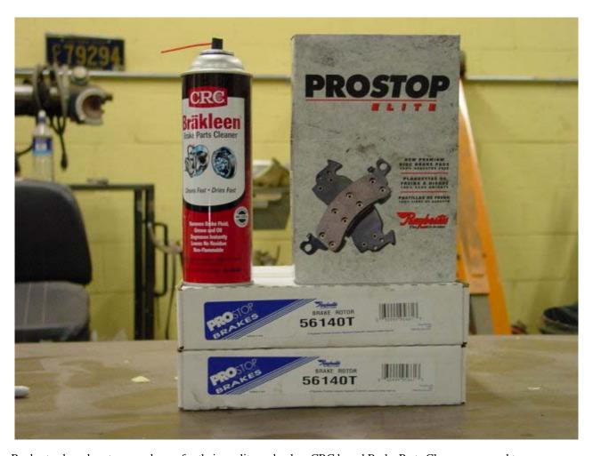
Raybestos brand parts were chosen for their quality and value. CRC brand Brake Parts Cleaner was used to remove any trace of machine oil from the new rotors.
