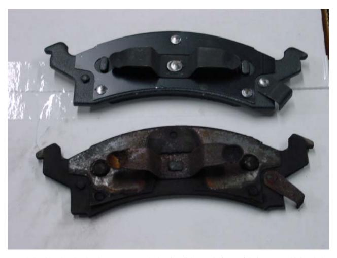
8. Match the old outboard pad to the new one. Note the location of the wear indicator. If the incorrect pad is installed (Right pad is installed on Left side) the wear indicator will not "chirp" when the pads are worn.
