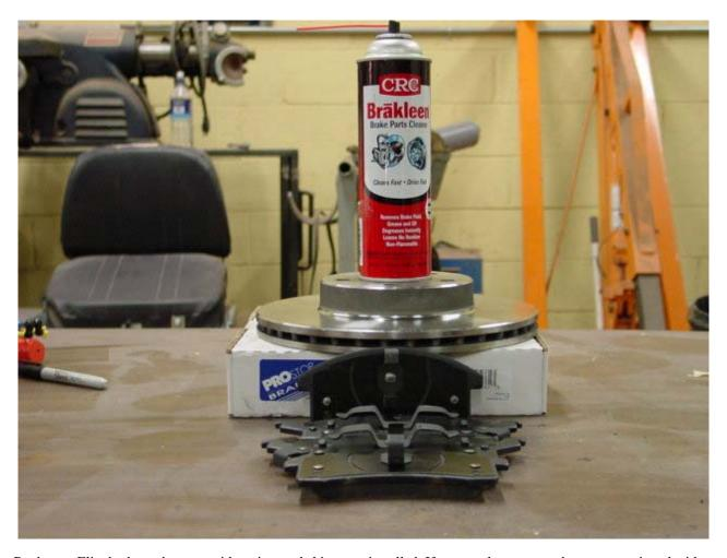
Raybestos Elite brake pads come with anti-squeal shims pre-installed. If your replacement pads are not equipped with shims, ask your parts counterperson about a shim kit. Many brake parts manufacturers sell shim kits. Its usually a better value to buy the pads with shims installed, as opposed to buying a shim kit and a set of brake pads.
