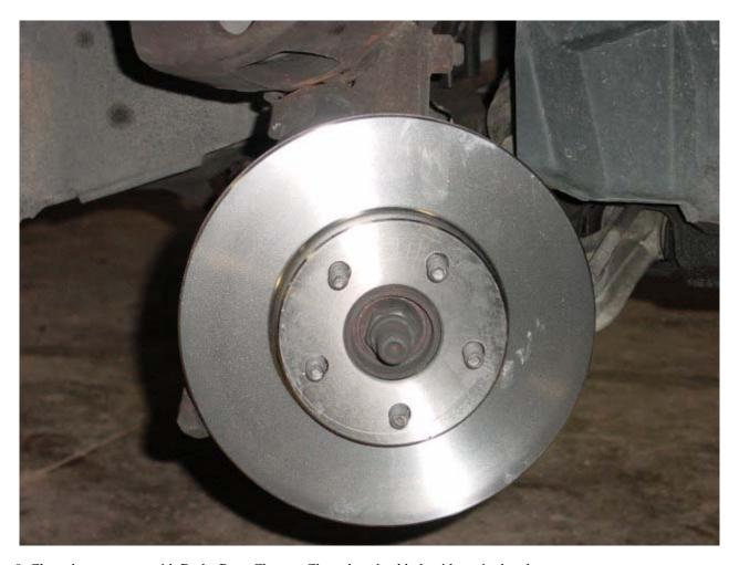
9. Clean the new rotor with Brake Parts Cleaner. Clean the wheel hub with a wire brush to remove any rust or corrosion. Install the new rotor.
