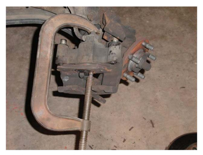
5. Using a large C-clamp, compress the caliper piston.
