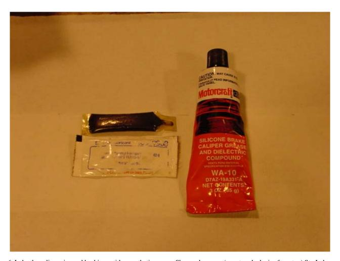
6. Lube the caliper pins and bushings with a synthetic grease. Shown above are (counter-clockwise from top) Sta-Lube Synthetic Brake Caliper Grease, GM Silicone Lubricant (in white packet) and Motorcraft Silicone Brake Caliper Grease and Dielectric Compound. Any of the above are acceptable. **DO NOT** use petroleum based grease. Petroleum based grease can cause the caliper bushings to swell. This binds the caliper and causes premature brake pad wear.
