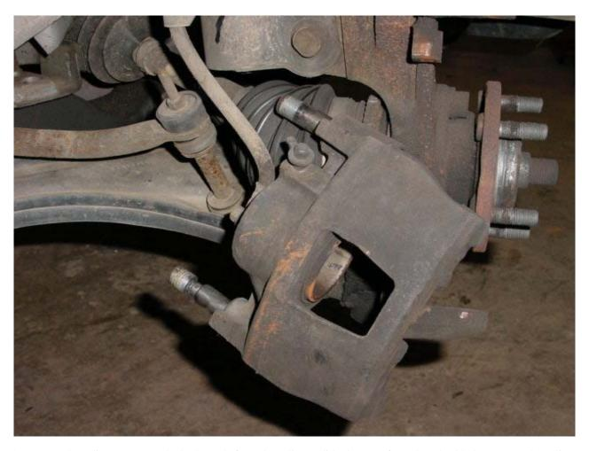
4. Remove the caliper. Remove the brake pads from the caliper. Slide the rotor from the wheel hub. Remove the caliper pins from their bores. Inspect the caliper pin bushings, caliper piston dust seal and the flexible brake hose for wear or damage. Replace worn or damaged parts.
