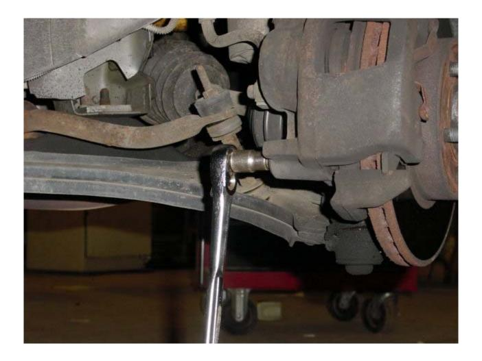
3. Remove the caliper bolts. In this instance, a 3/8" Allen head socket is needed. Other cars may use a Torx head fastener or a conventional hex bolt.
