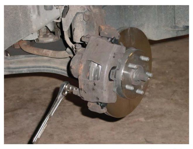
10. Install the new pads on the caliper, then install the caliper. Torque the caliper pins to manufacturer's specification. Clean the rotor once again with Brake Parts Cleaner to remove any fingerprints or traces of oil/grease.
