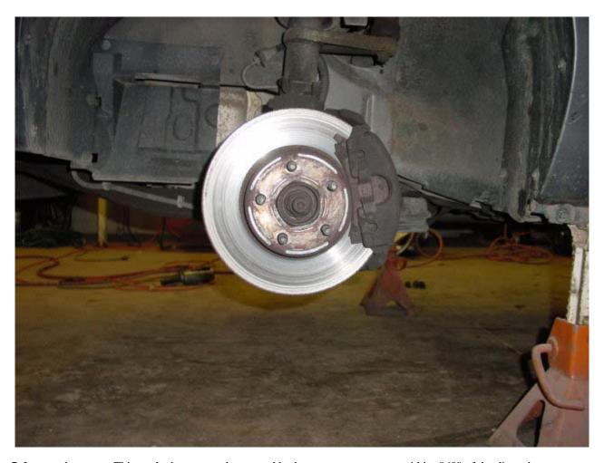
7. Inspect the rotors. This car had one scored rotor and both rotors were worn to within .060" of the discard specification. Both rotors also measured .009" runout, which caused a nasty vibration when braking. While the rotors could have been saved via machining, the owner opted to install new rotors for years of trouble-free braking.
