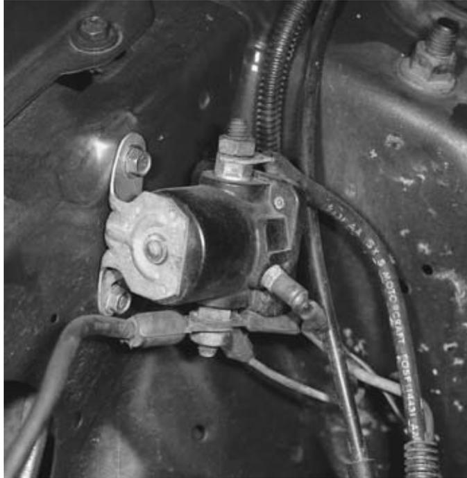
Figure 9-12. The Ford starter relay or magnetic switch.
