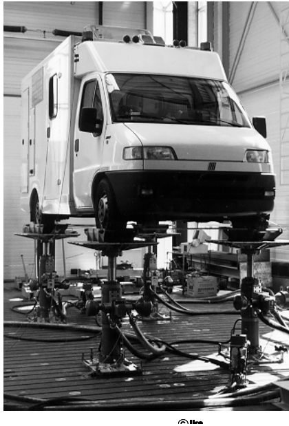
Fig.1.7-5: 4-cylinder servo-hydraulic test bench
