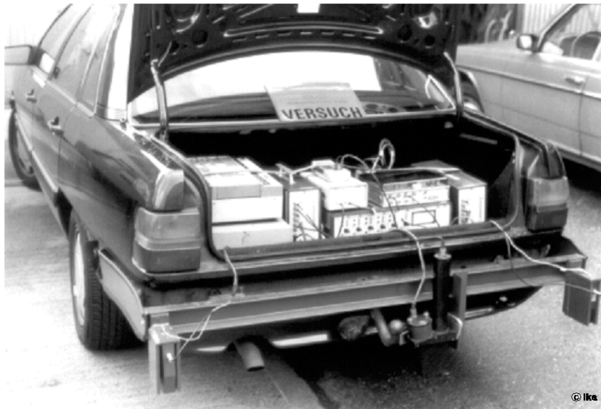
Fig. 1.2-6: Instrumentation for unevenness measurements (ika)
