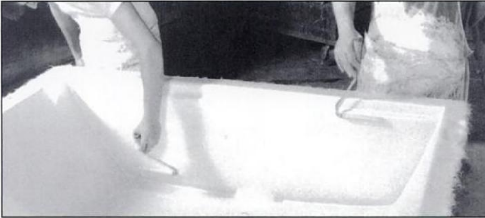
Especially when mat is used, each layer of laminate must again be consolidated by rolling. Photo courtesy FRP Supply Division, Ashland Chemical Co.
