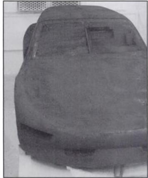
To protect the foam from attack by the polyester resin in body filler, it is sprayed with exterior latex house paint. The surface can now have body filler applied.
