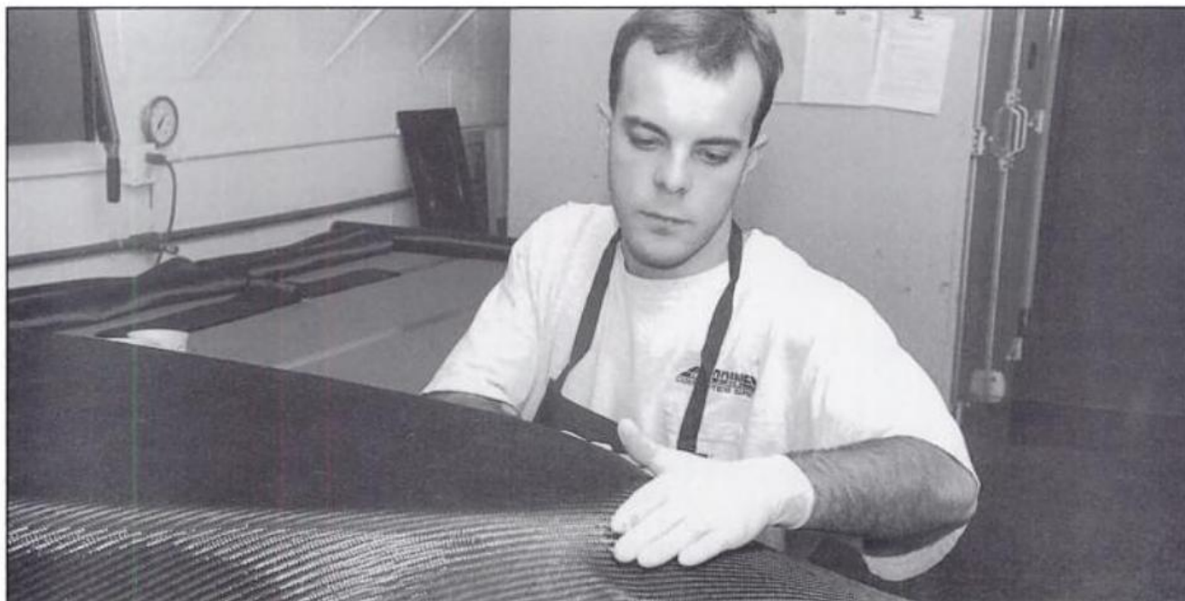
Reinforcement can be urged into place with a gloved hand. Photo by Jack Gladback.
