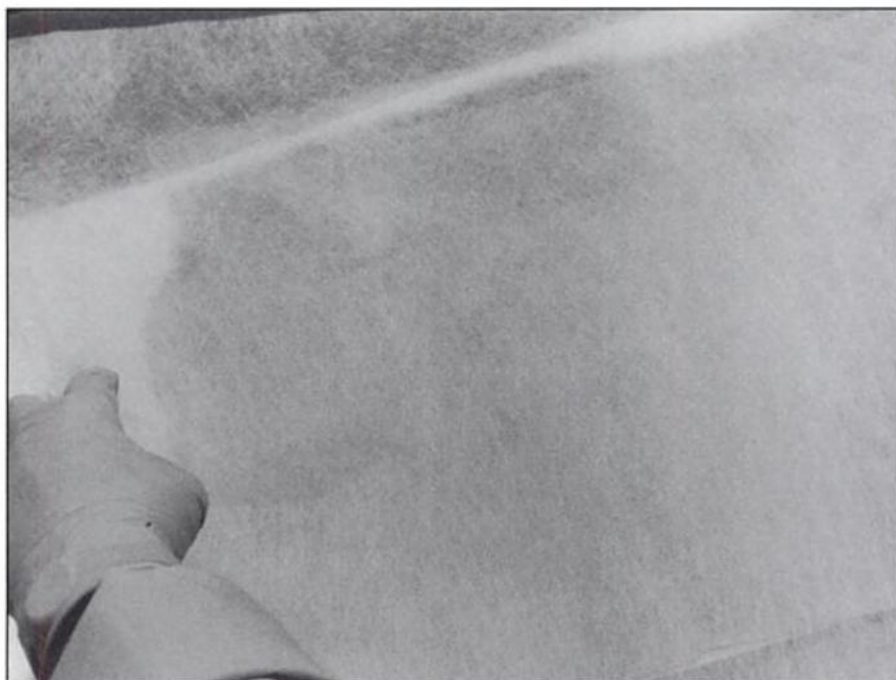
Surfacing veil looks like very thin mat. It is sometimes used as a cover to prevent print-through of fabric weave. Photo courtesy DOW Plastics.
