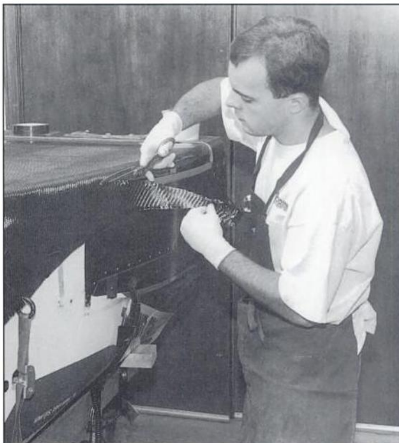
With careful timing, and luck, laminates at a green cure stage can be trimmed in or on the mold. This saves much difficult and messy cutting of fully-cured laminate. Photo by Jack Gladback.
