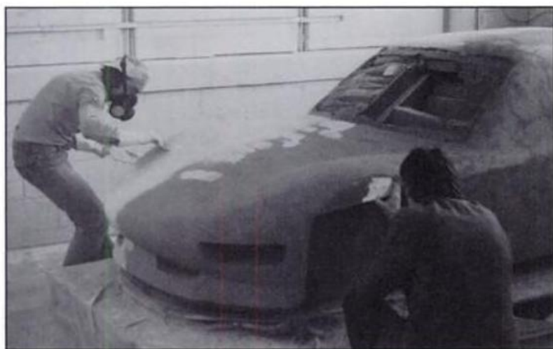
Repeated sanding and painting is needed, as well as countless local repairs with spot putty. This work can prove gruelling.
