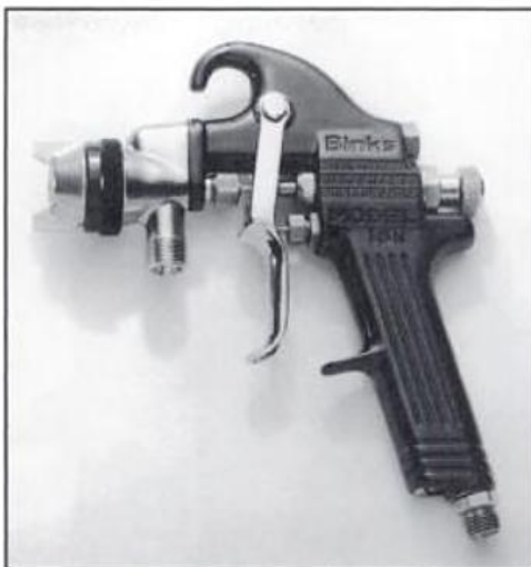
A catalyst injection type gun. The catalyst flows through the "ears" for atomizing air. Photo courtesy Binks Manufacturing Co.
