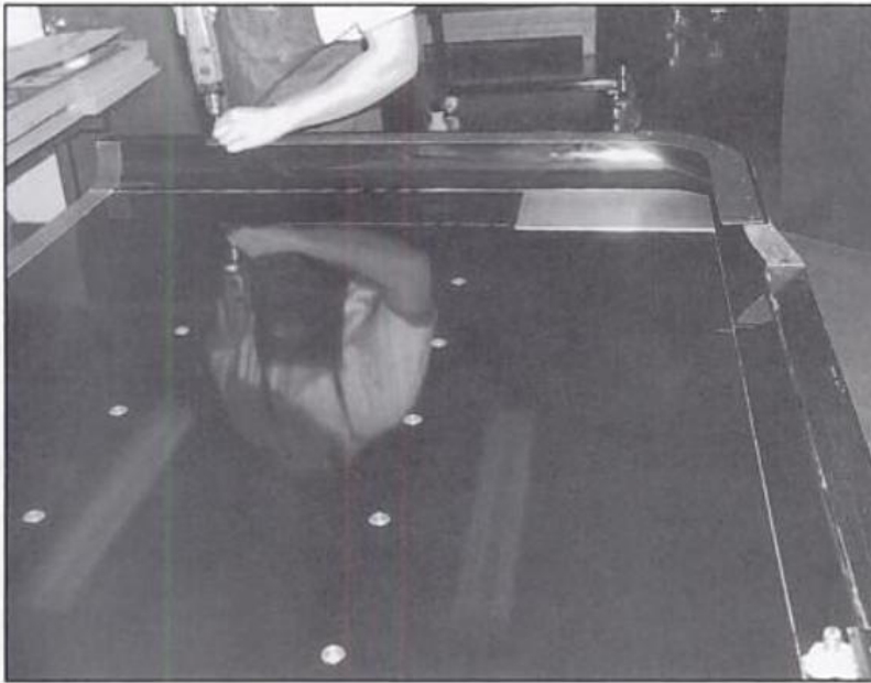
Large flat areas are best avoided in FRP construction, because such shapes lack the inherent stiffness of curved panels. Photo by Jack Gladback.
