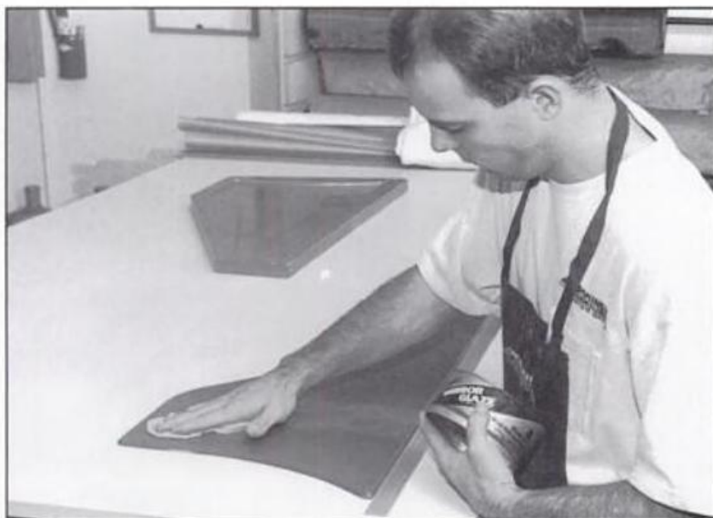
The most common parting agent (mold release) is wax. On small parts, this is most conveniently applied by hand. Photo by Jack Gladback.
