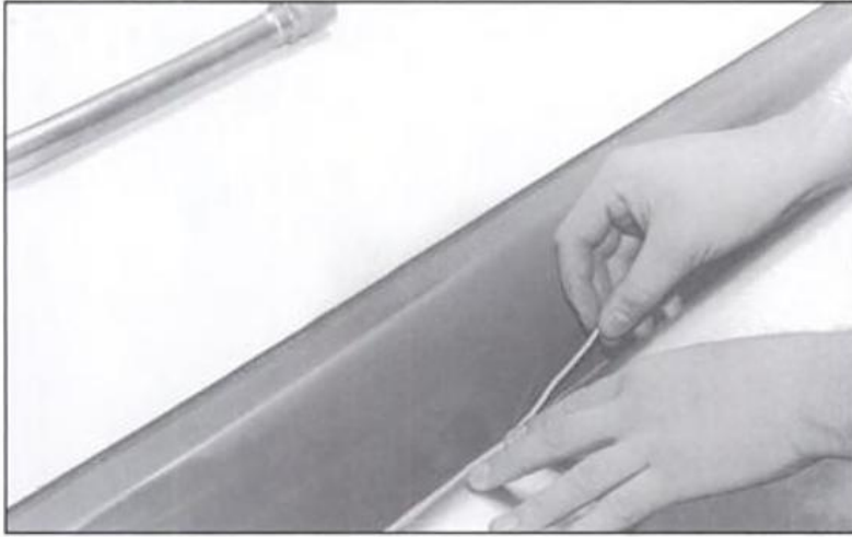
Sharp corners are also best avoided in FRP. Sometimes it is easiest to produce a plug with "square" corners, then form a radius before mold making using a fillet of wax or modeling clay. Photo by Jack Gladback.
