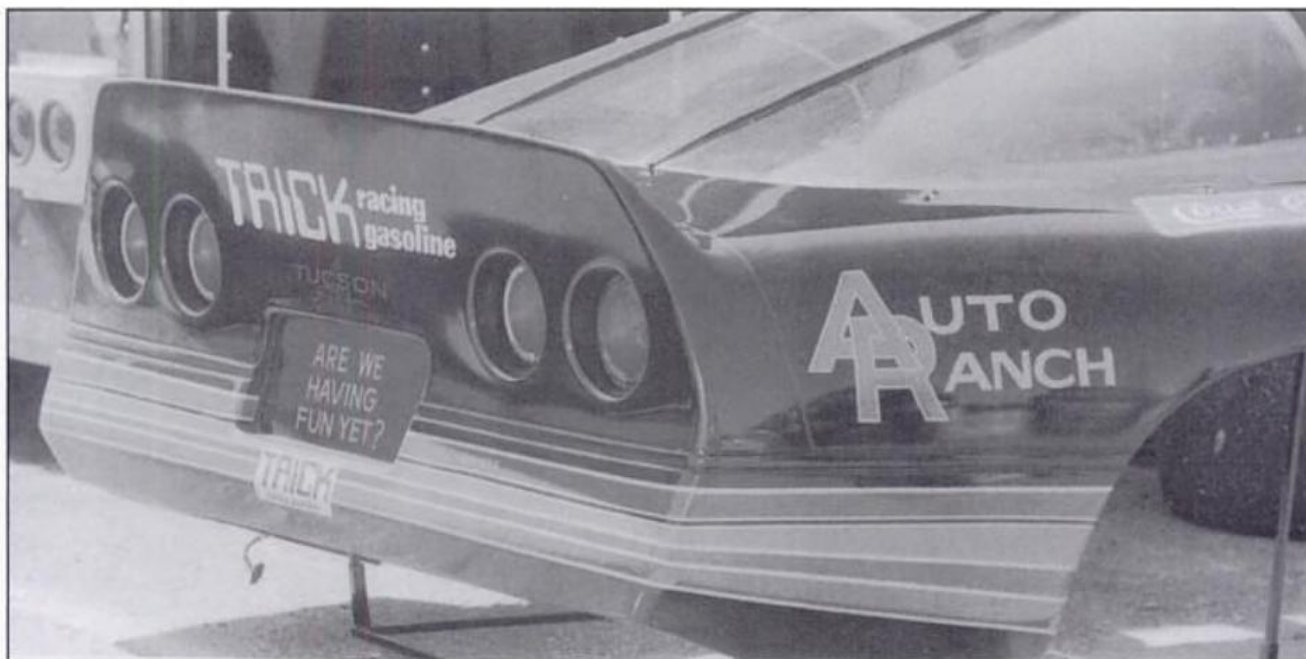
Race car body parts such as these will need multi-piece molds. Photo by Michael Lutfy.
