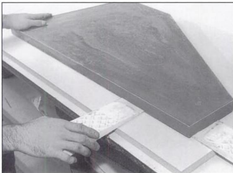
Nylon wedges sometimes aid separation of mold and part. If this doesn't work, more drastic measures will have to be taken. Photo by Jack Gladback.
