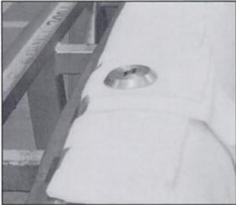
Note use of additional bleeder ply at vacuum connections to prevent resin entering vacuum system. Guy Levesque photo courtesy deHavilland Inc.
