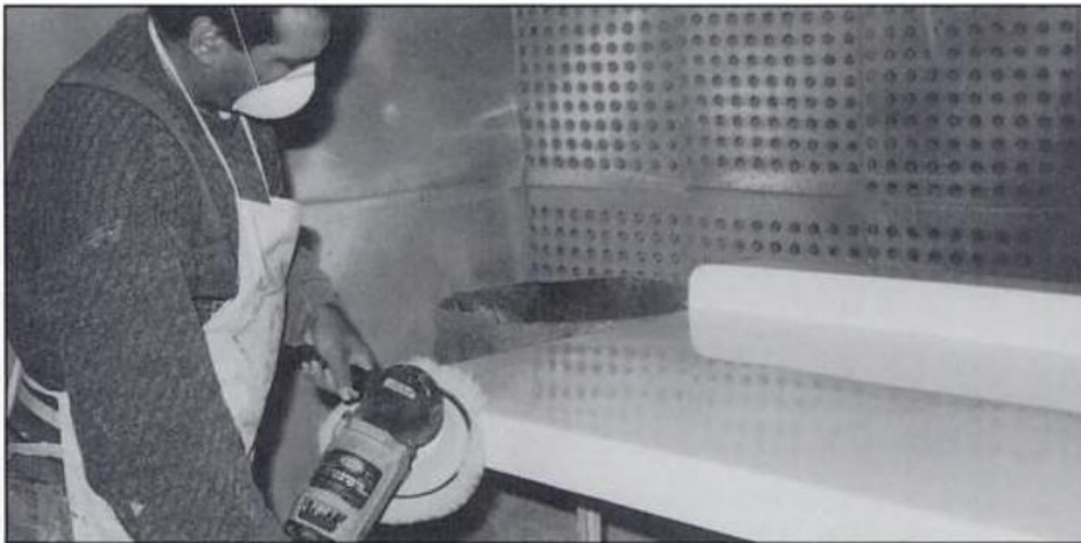
This shop worker almost gets an "A" for his protective gear. He's got the mask, an apron (gloves aren't really necessary here) but he's missing eye protection. Photo by Michael Lutfy.
