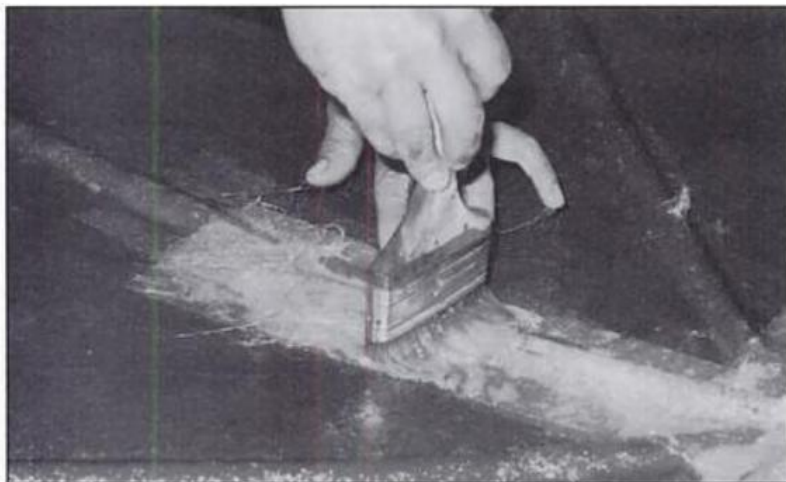
When applying more resin, use a paint brush but don't "brush," like shown above. Use a poking or "stippling" motion to coat the mat. Photo by Michael Lutfy.
