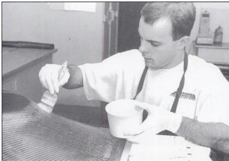
Additional resin to ensure complete saturation can then be applied by brush. Photo by Jack Gladback.
