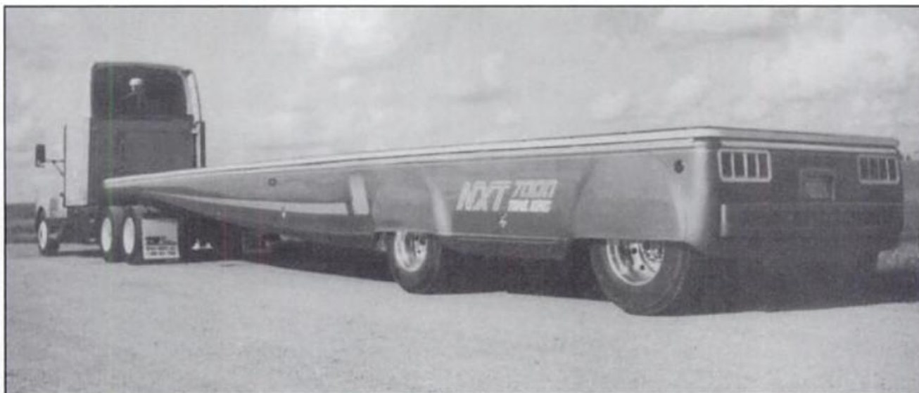
Large trailer beds can be lightened considerably with FRP construction. This, of course, helps to improve fuel economy. Photo courtesy Escom Advertising Group, Inc.
