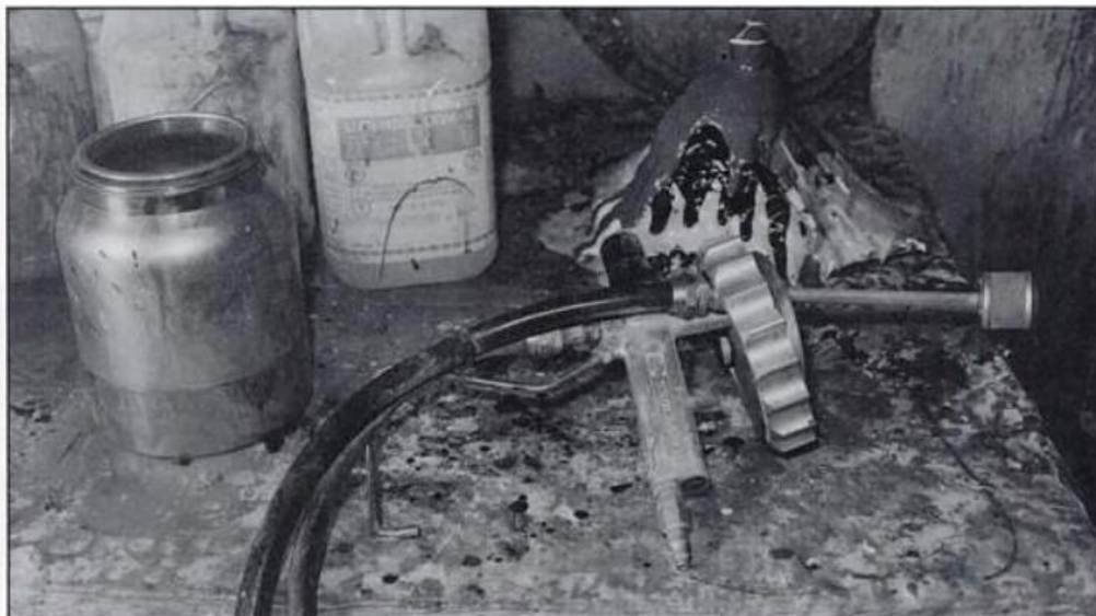
The tools of the gel coat sprayer's trade. This bench in the gel coat spray booth of a boat builder has obviously seen some heavy use. Note the "volcano" of gel coat growing in the back. Photo by Michael Lutfy.
