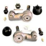
**Step 1** Always buy name-brand tie-rod ends. Also beware that each side is threaded differently, so the part numbers should be different. Ask the parts person to label left and right.
