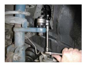
**Step 2** With the vehicle raised, secured, and its front wheels removed, begin the tie-rod-end job by loosening the pinch bolt on the end itself or on the adjuster sleeve (depending on end style).
