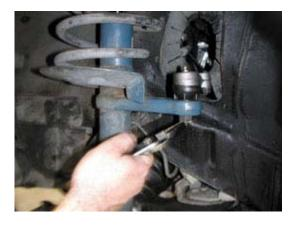
**Step 4** Use a 2-jaw or tie-rod puller (shown) to disconnect the end.
