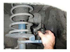
**Step 6** Install the new rubber boots on the replacement tie-rod ends and then reverse the disassembly procedure. Always use the new hardware and cotter pins that come with the replacement ends and torque all fasteners to factory spec.
