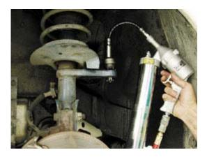
**Step 7** Lube the new ends until the grease seeps from behind the boots. Then wipe off any excess external grease.
