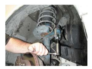
**Step 5** Before unscrewing the old ends, mark their positions so the new ones can be installed in roughly the same positions. Install the grease fittings into the new ends, if applicable.
